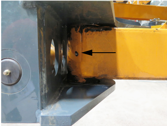
Main Fold Pivot Grease Zerk - Lower (2) -Typical View
