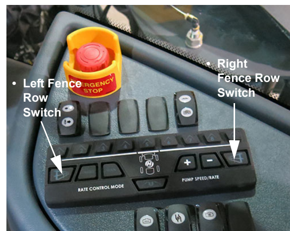
Fence Row Switches - Left and Right (Located on the side console) -Typical View
