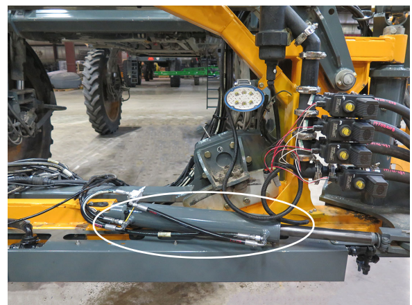
Main Fold/Breakaway Cylinder -Typical View
