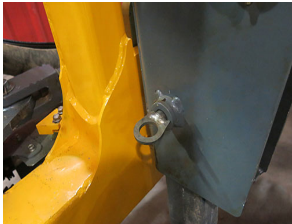
Lock Pin Removed -Typical View
