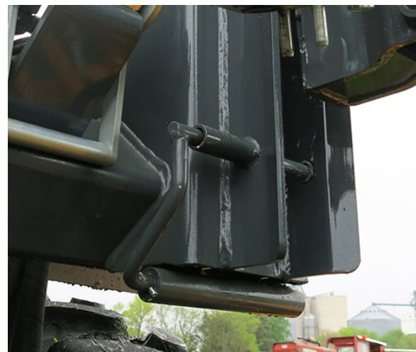
Lock Pin (2) -Typical View * Engaged position shown
