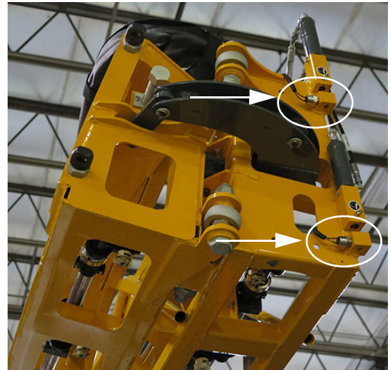
Outer Fold Latch Sensors (4) -Typical View
