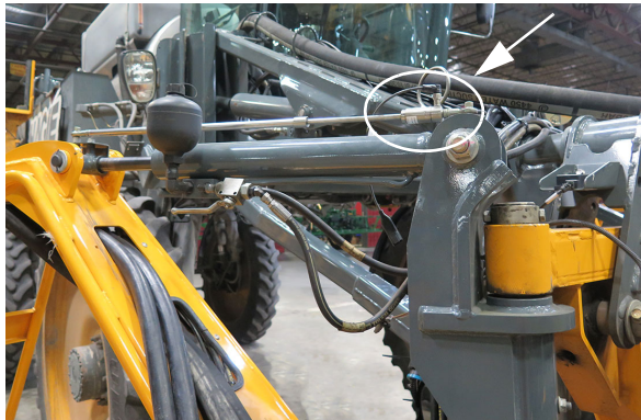
Position Sensor (2) -Typical View
