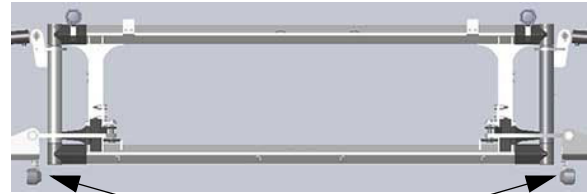
Night Spray Lights (2) (Located on each side of the main boom fold section) -Typical View
