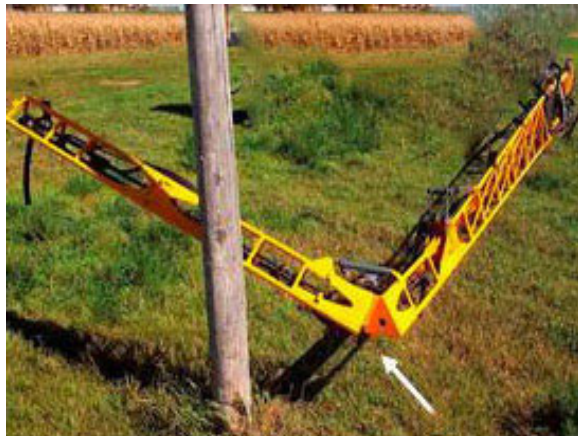
Outer Boom Breakaway -Typical View
