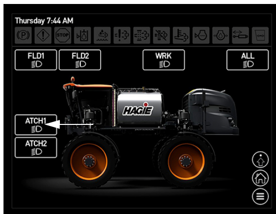
Attachment Lights Button (ATCH1) (Located on the Machine Display Exterior Lighting Screen)
