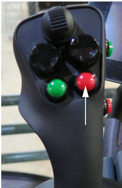
End Row Management Switch (Located on the Hydrostatic Drive Control Handle) -Typical View
