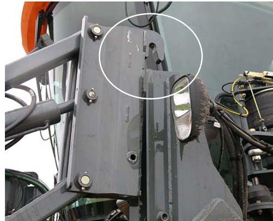
Attachment Clearing Mounting Pin -Typical View
