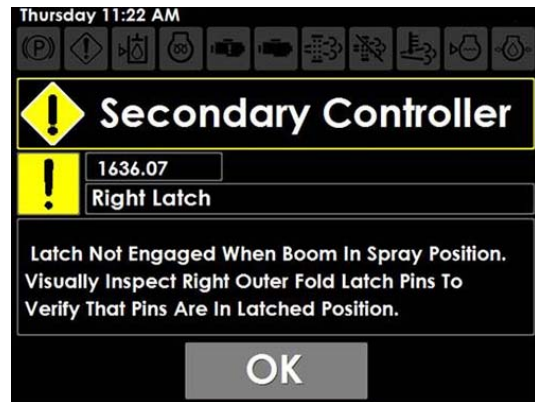
Outer Fold Latch "Not Engaged" Malfunction Warning
