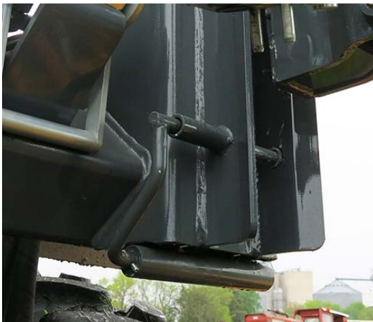
Lock Pin -Typical View * Engaged position shown
