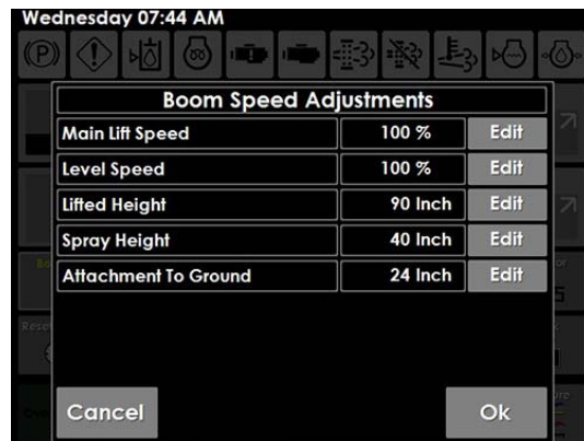
Boom Speed Adjustments Screen (Located on the Settings Page)
