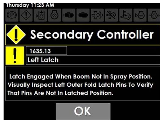
Outer Fold Latch "Engaged" Malfunction Warning
