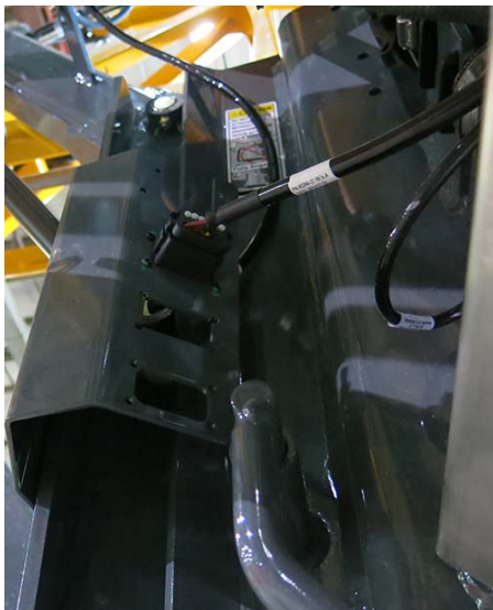
NORAC Connection - if equipped (Located on the front right-hand side of machine) -Typical View
