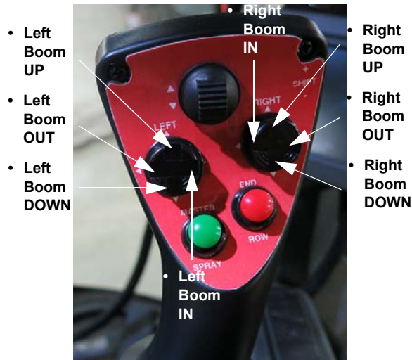
Left and Right-Hand Boom Switches (Located on the Hydrostatic Drive Control Handle) -Typical View
