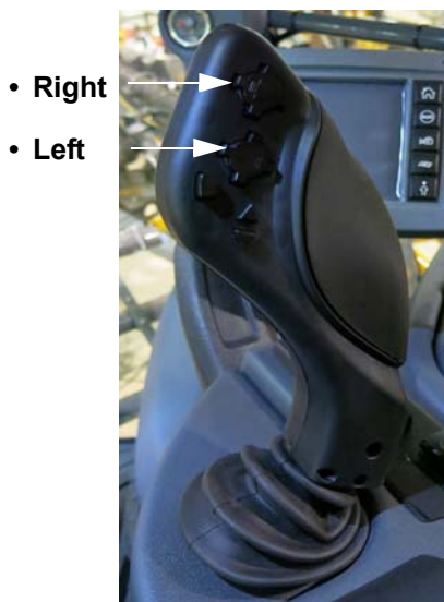
Left and Right Boom Switches (Located on the Hydrostatic Drive Control Handle) -Typical View
