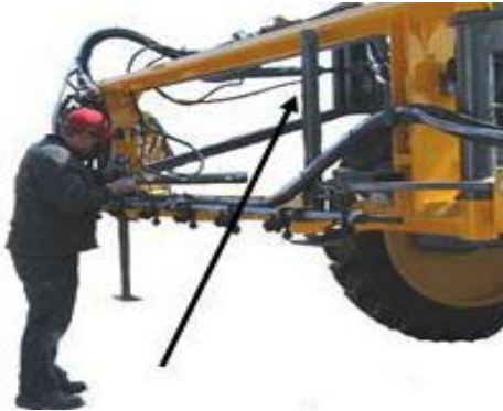
Boom Stand in “Travel” Position -Typical View
