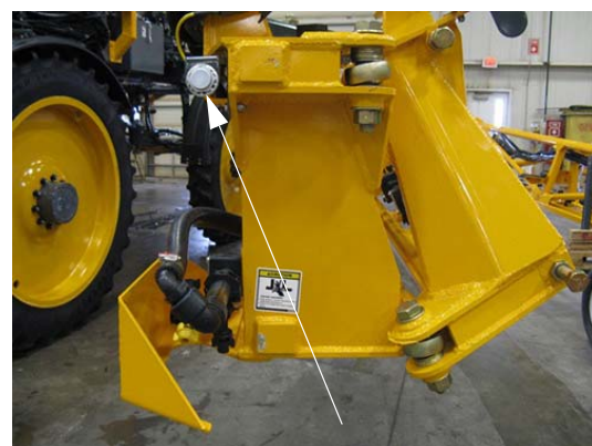
Proximity Sensors -Typical View
