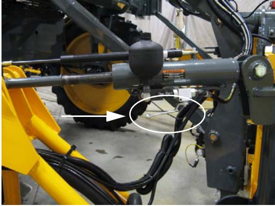
NORAC Hand Valve (2) - if equipped (Located on the left and right-hand level cylinders) -Typical View * Right-hand level cylinder shown
