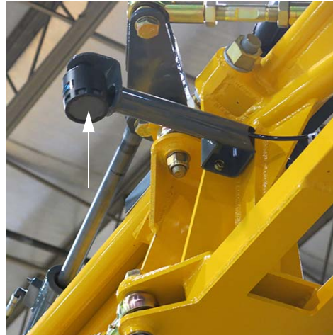
Norac Sensor Foam Pad (Located on the bottom of each Norac Sensor) -Typical View
