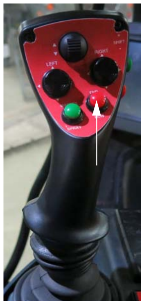
End Row Management Switch (Located on the Hydrostatic Drive Control Handle - Version 2) -Typical View
