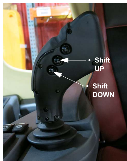
Shift Up/Down Switches (Located on the back side of the Hydrostatic Drive Control Handle - Version 1) -Typical View
