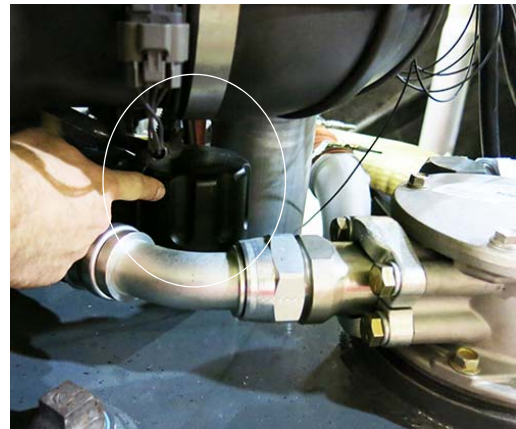
Breather Cap (Located on left-hand side of machine near return filter housing) -Typical View
