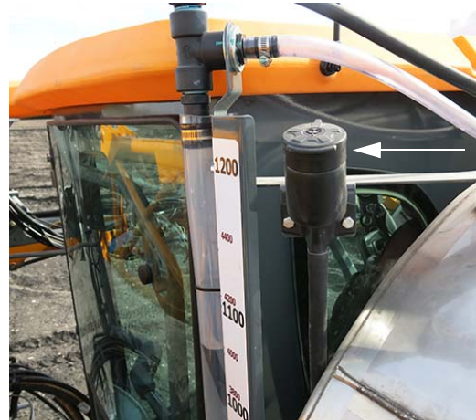
Windshield Washer Fluid Reservoir (Located behind the left-hand side of cab) -Typical View
