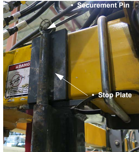
Stop Plate/Securement Pin Assembly -Typical View
