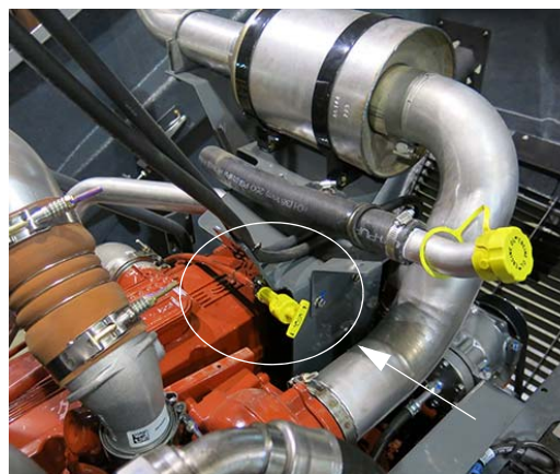
Engine Oil Dipstick (Located on rear left-hand side of machine - open hood to access) -Typical View
