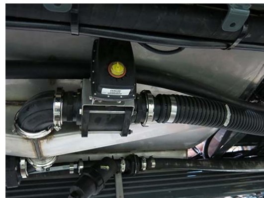
Solution Tank Valve -Typical View
