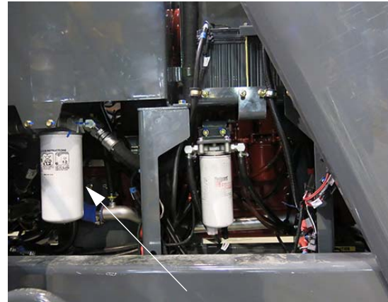
Case Drain Filter (Located on left-hand side of machine - open hood to access) -Typical View
