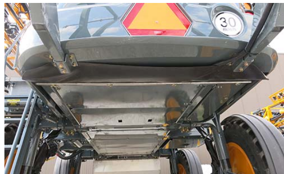
Belly Shield/Brush Curtain Installation -Typical View
