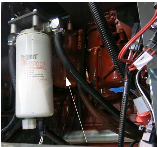
Engine Oil Filter (Located along the left-hand side of machine - open hood to access) -Typical View
