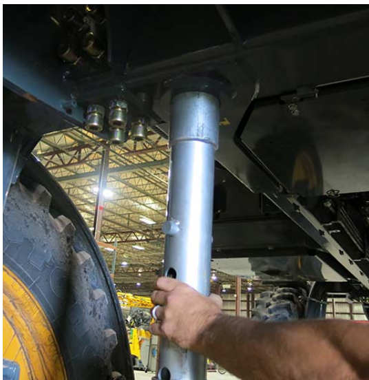
Insert Jack into Lifting Point Containment Ring -Typical View
