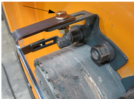
Hub Cap Adapter Bolt Installation -Typical View
