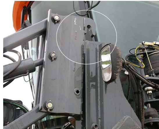
Attachment Clearing Mounting Pin -Typical View
