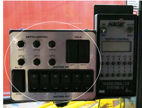
Detasseling Control Panel -Typical View
