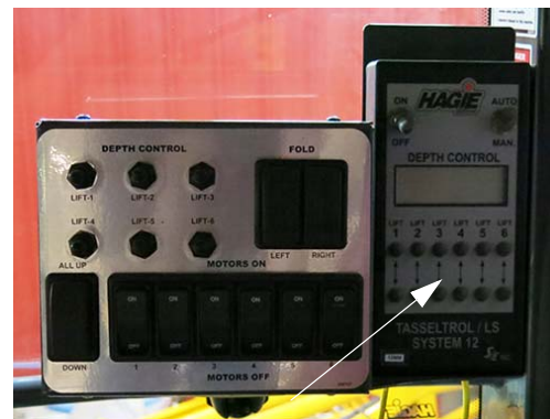
Tasselrol/LS System 12 Control Panel -Typical View
