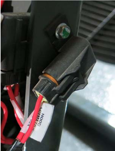
Hood Actuator Fuse (Located near rear left-hand side of machine) -Typical View
