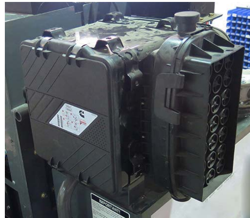
Engine Air Intake Filter (Located along catwalk on left-hand side of machine - open hood to access) -Typical View
