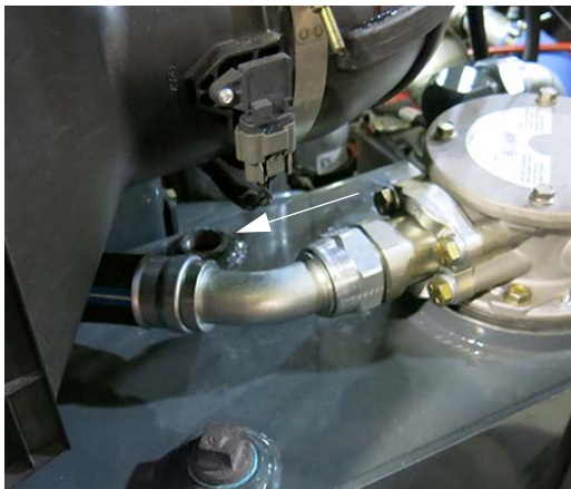
Breather Cap Removed -Typical View
