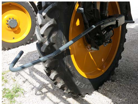
Installed Crop Divider -Typical View
