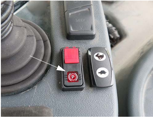
Parking Brake Switch - if equipped (Located near the Hydrostatic Drive Control Handle) -Typical View
