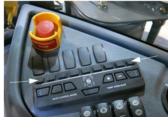
Boom Solution Valve Switches - Sections 1 and 9 (Located on the side console) -Typical View
