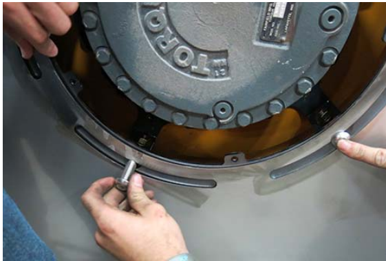
Wheel Cover Mounting Bolt Installation -Typical View
