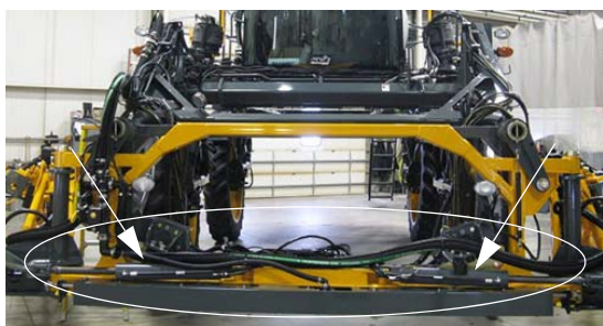
Main Pivot/Breakaway Cylinders -Typical View
