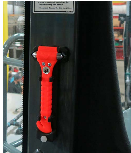
Emergency Exit Tool (Located along rear right-hand side of cab) -Typical View
