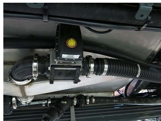
Solution Tank Valve -Typical View
