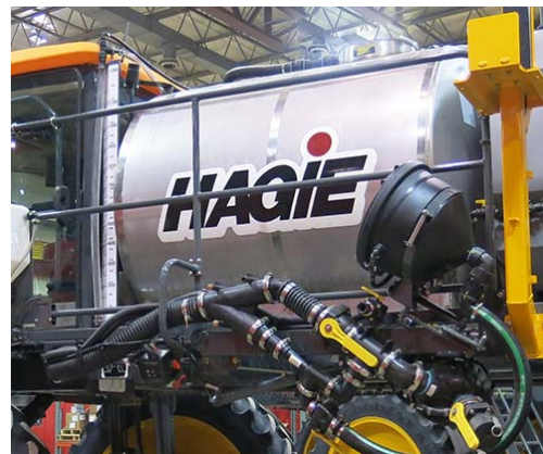
Solution Tank -Typical View
