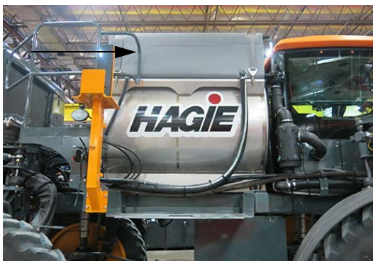
Rinse Tank -Typical View
