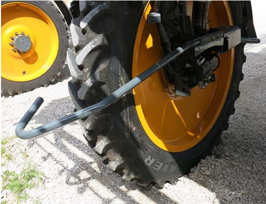
Installed Crop Divider -Typical View
