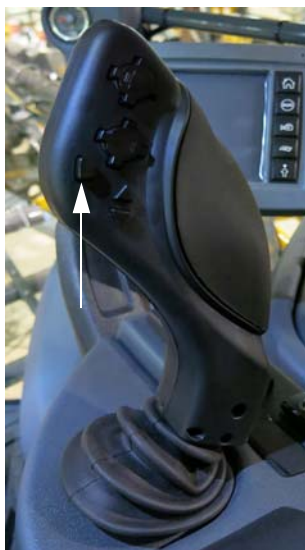
End Row Management Switch (Located on the Hydrostatic Drive Control Handle - Version 1) -Typical View
