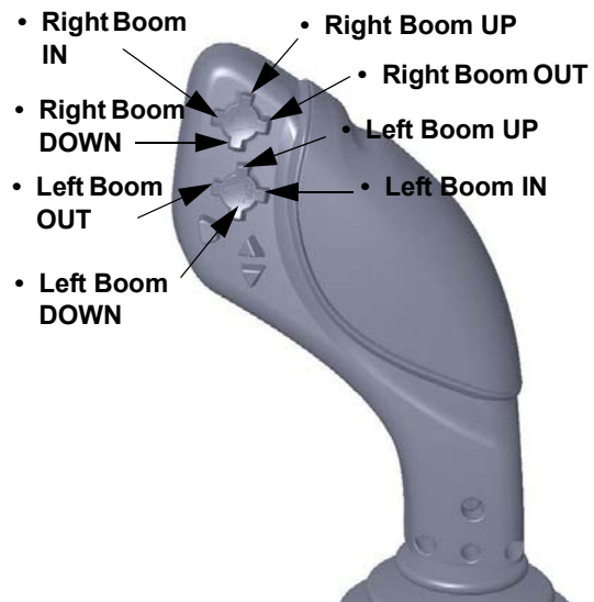
Left and Right-Hand Boom Switches (Located on the Hydrostatic Drive Control Handle - Version 1) -Typical View
