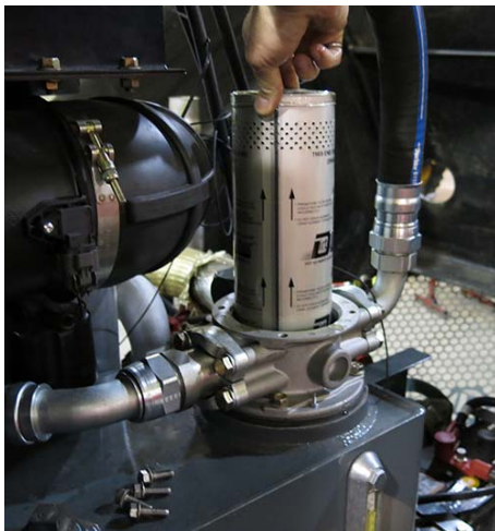
Return Filter (Located inside filter housing on left-hand side of machine) -Typical View
