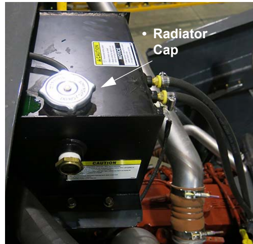
Radiator (Located near the rear of machine - open hood to access) -Typical View
