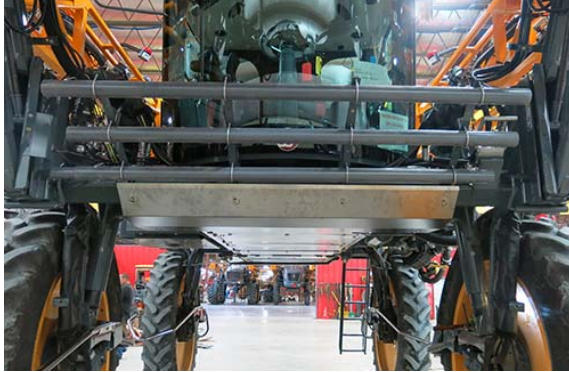
Brush Guard Installation -Typical View
