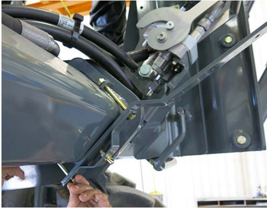
Anchor Bolt Assembly -Typical View
