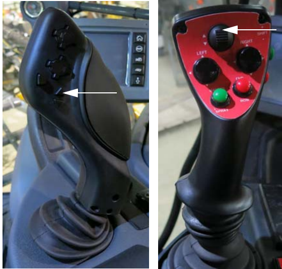
Transom Switch - UP (Located on the Hydrostatic Drive Control Handle) -Typical View
