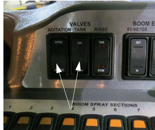
Tank and Agitation Valve Switches (Located on the side console) -Typical View
