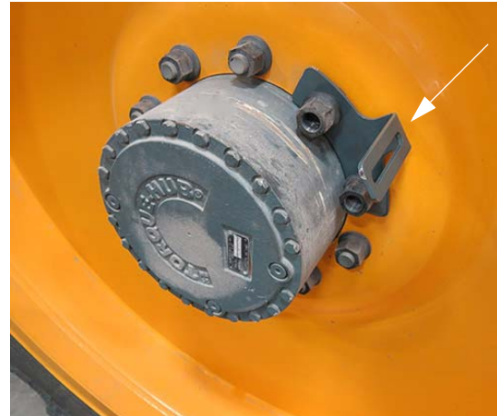
Hub Cap Adapter Plate -Typical View
