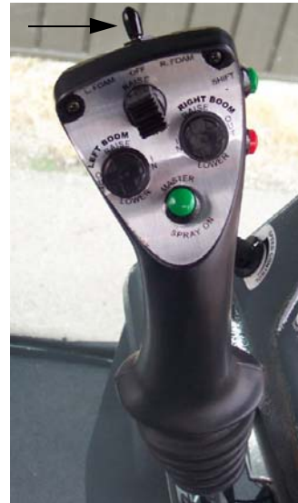
Foam Marker Switch (Located on the Hydrostatic Drive Control Handle) -Typical View
