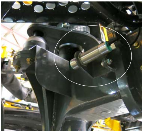
Tread Adjust Electronic Sensors (Rear Legs) -Typical View
