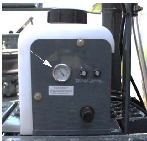
Foam Marker Pressure Gauge (Located on the side of the fill tank) -Typical View
