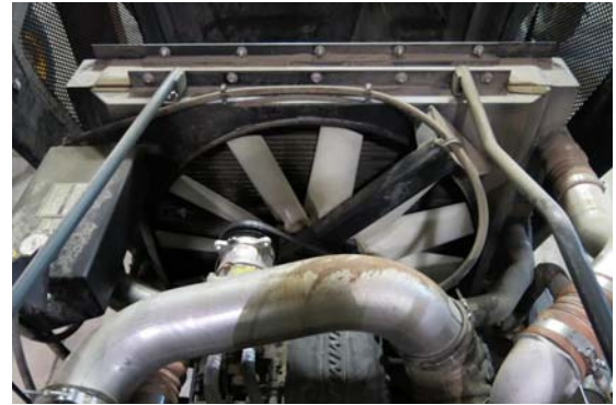
Reversible Fan (Located near rear of machine - open hood to access) -Typical View
