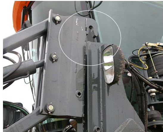
Attachment Clearing Mounting Pin -Typical View
