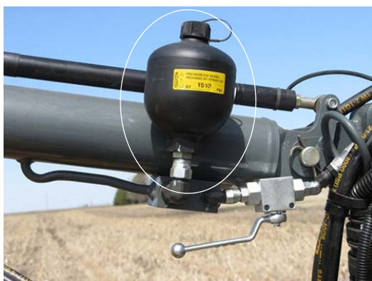
Accumulator -Typical View
