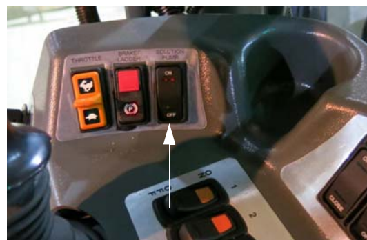
Solution Pump Switch (Located on the side console) -Typical View
