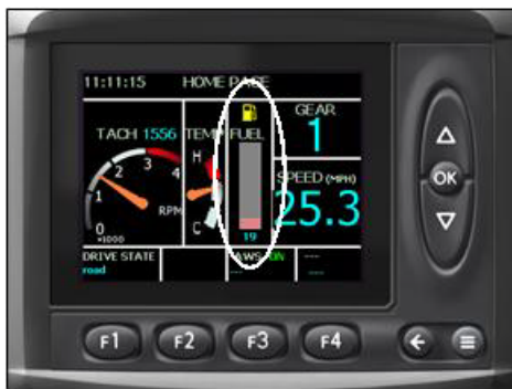
Fuel Gauge (Located on the Home Page) -Typical View
