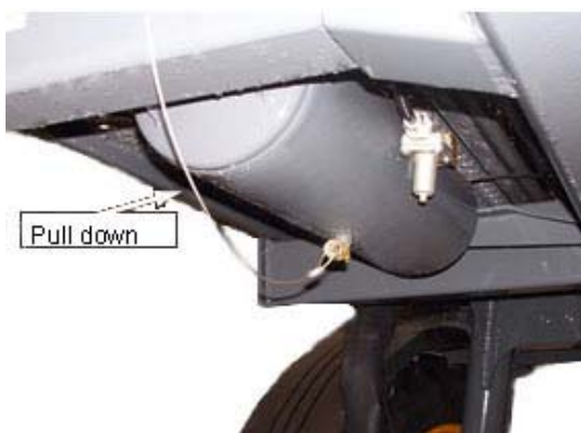
Air Tank Drain Valve (Located beneath catwalk on left-hand side of machine) * Pull DOWN to open -Typical View
