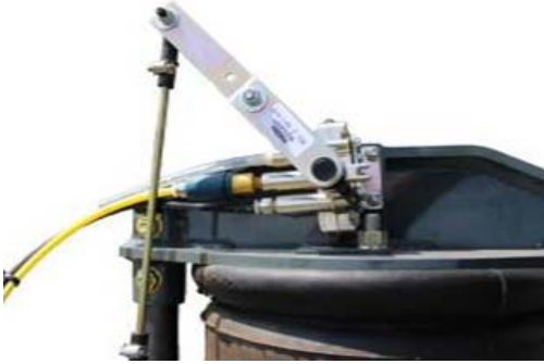
Dump Valve (One valve located on each leg) -Typical View
