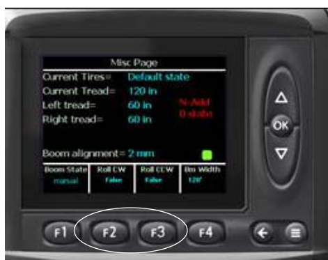
F2/F3 Switches - Roll Command (Located on the MD3 Monitor - Misc Page) -Typical View
