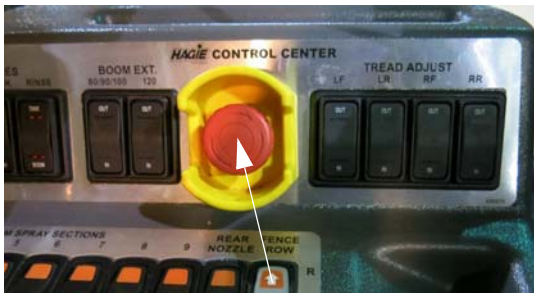
Emergency Stop Switch (Located on the side console) -Typical View
