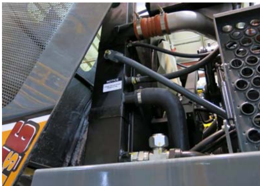
A/C Charge Port (Located on right-hand side of machine - open hood to access) -Typical View
