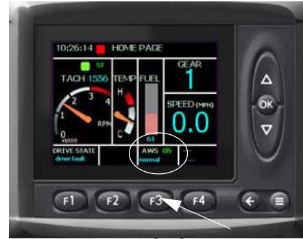
F3 (AWS) Switch (Located on the MD3 Monitor) -Typical View
