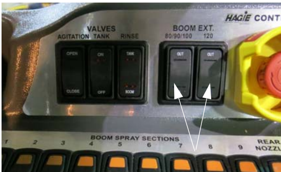
Boom Extension Switches (Located on the side console) -Typical View
