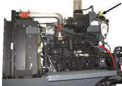
Engine Oil Dipstick (Located on the left-hand side of engine) -Typical View
