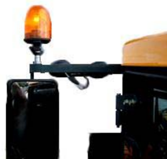
Rotating Beacon (Located on the left-hand side of the operator's station) -Typical View
