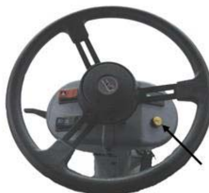
Horn Button (Located on the right-hand side of the steering column) -Typical View
