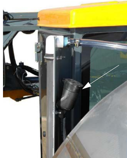
Windshield Washer Fluid Reservoir (Located behind the left-hand side of cab) -Typical View
