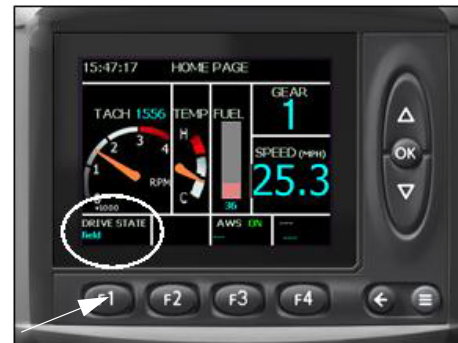
F1 (Drive State) Switch (Located on the MD3 Monitor) -Typical View
