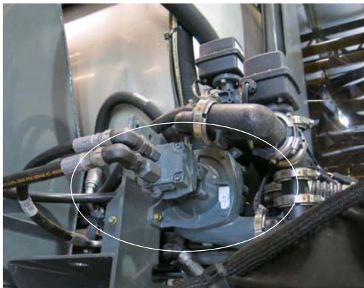
Solution Pump (Located near front right-hand side of machine) -Typical View
