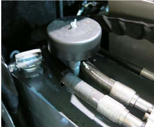
Breather Cap (Located on top of hydraulic oil reservoir - open hood to access) -Typical View
