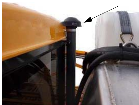
Fresh Air Tube (Located behind the cab) -Typical View
