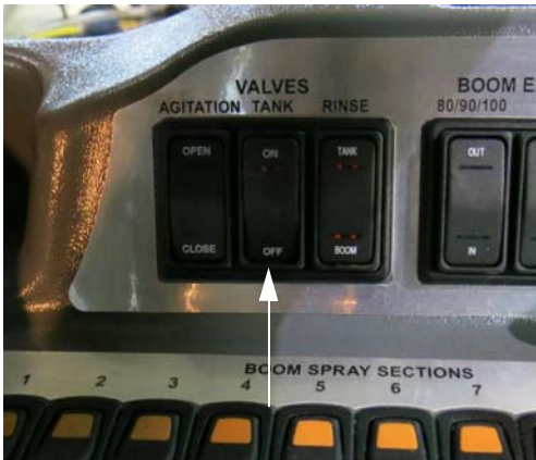
Tank Valve Switch (Located on the side console) -Typical View
