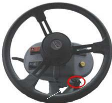
Ignition Switch (Located on the right-hand side of the steering column) -Typical View
