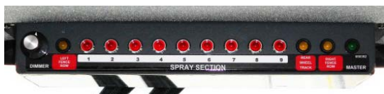
Boom Solution Valve LED Indicators -Typical View
