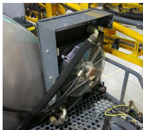
Auxiliary Hydraulic Cooling Fan (Located behind solution tank on the right-hand side of machine) -Typical View
