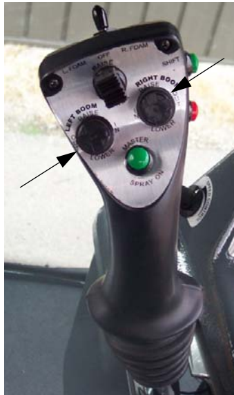
Left/Right Boom Switches (Located on the Hydrostatic Drive Control Handle) -Typical View
