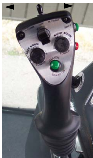
Foam Marker Switch (Located on the Hydrostatic Drive Control Handle) -Typical View
