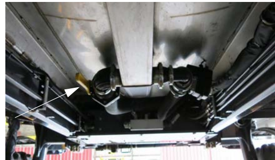
Sump Valve (Located beneath the solution tank) -Typical View
