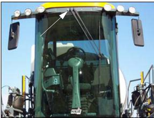
Windshield Washer Fluid Spray Nozzle (Located near top of exterior cab) -Typical View
