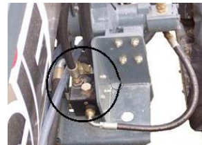
Pulse Width Modulated Valve -Typical View
