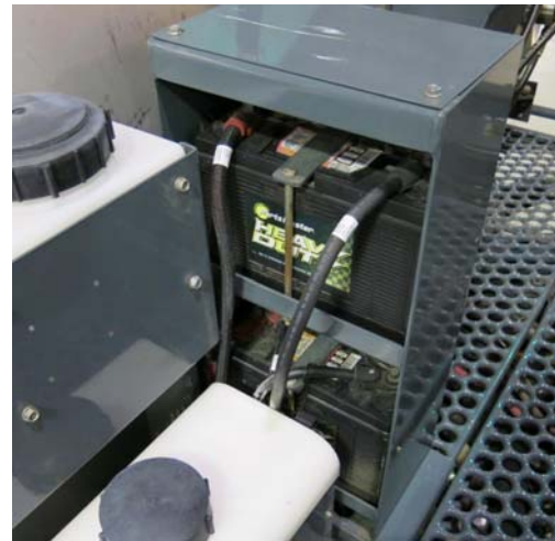
Battery Access (Located at rear of machine - remove panel to access) -Typical View
