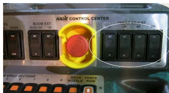
Tread Adjust Switches (Located on the side console) -Typical View
