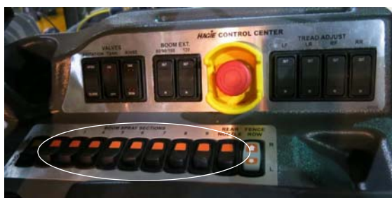
Boom Solution Valve Switches (Located on the side console) -Typical View
