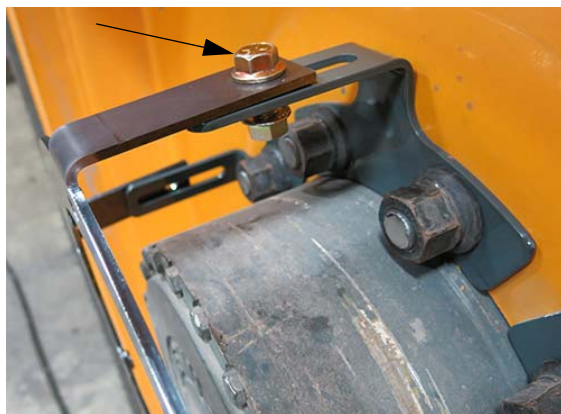
Hub Cap Adapter Bolt Installation -Typical View
