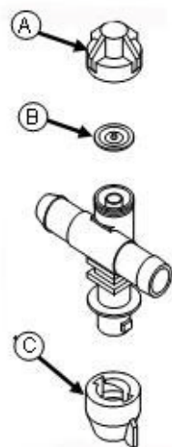
Nozzle Diaphragms and Spray Tips -Typical View
