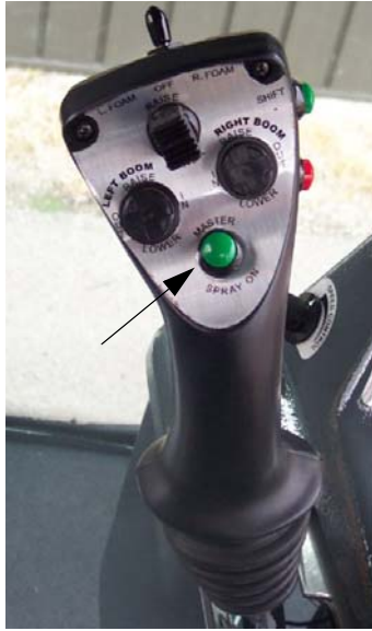
Master Spray Switch (Located on the Hydrostatic Drive Control Handle) -Typical View
