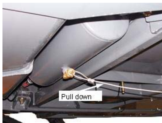
Wet Tank Drain Valve (Located beneath catwalk on left-hand side of machine) * Pull DOWN to open -Typical View
