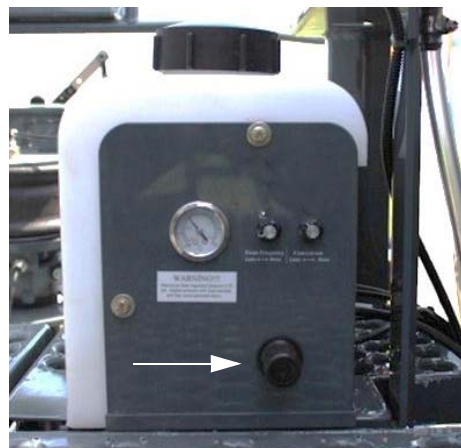
Foam Pressure Dial (Located on the side of the fill tank) -Typical View
