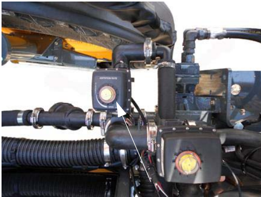
Variable Flow Solution Valve (Located near the solution pump) -Typical View
