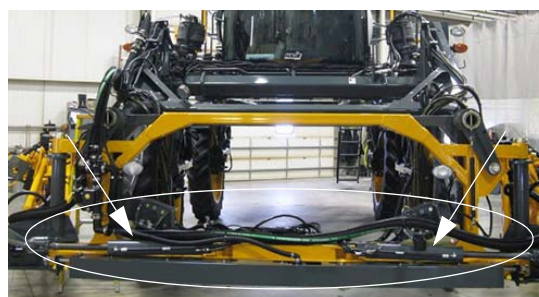
Main Pivot/Breakaway Cylinders -Typical View
