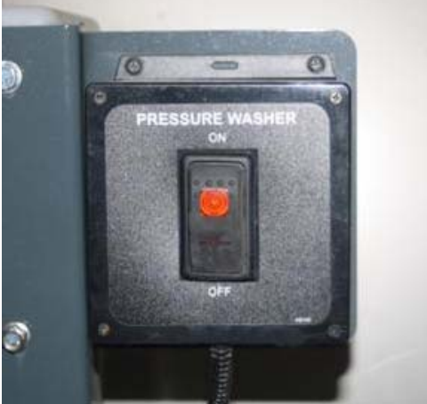
Pressure Washer Switch (Located on the side of the fresh water tank) -Typical View
