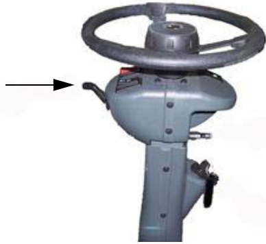
Turn Signal Lever (Located on the left-hand side of steering column) -Typical View
