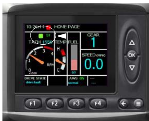
Spray Boom Indicator Light (Located on the MD3 Monitor - Home Page) -Typical View
