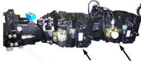
Tandem Hydrostatic Pumps -Typical View
