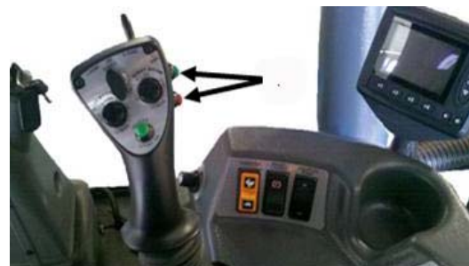
Speed Range Switches (Located on the side of the Hydrostatic Drive Control Handle) -Typical View
