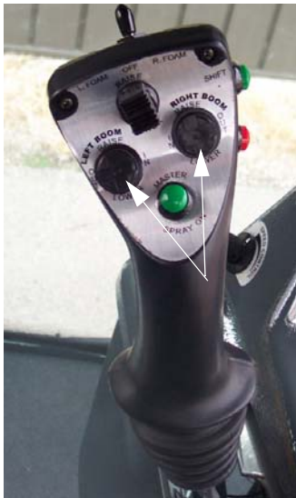
Left and Right Boom Switches (Located on the Hydrostatic Drive Control Handle) -Typical View
