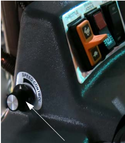
Speed Control Dial (Located on the side console) -Typical View
