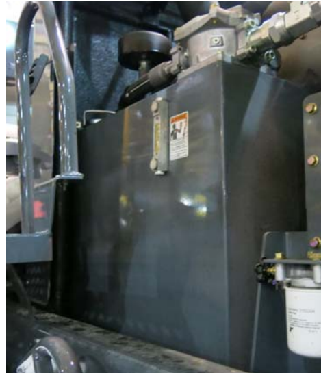
Hydraulic Oil Reservoir (Located on left-hand side of machine - open hood to access) -Typical View
