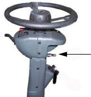
Steering Wheel Tilt Adjust Handle (Located on the right-hand side of the steering column) -Typical View
