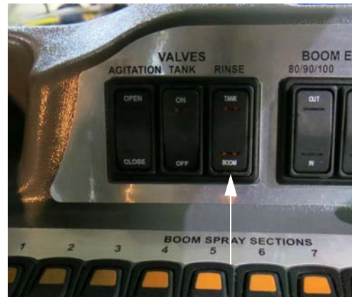
Rinse Switch (Located on the side console) -Typical View
