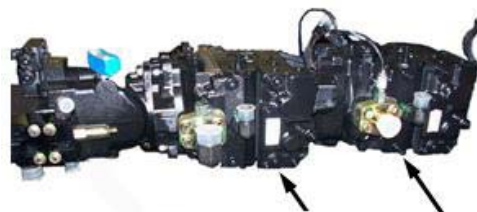
Tandem Hydrostatic Pumps -Typical View
