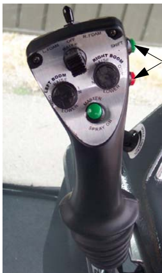
Speed Range Switches (Located on the side of the Hydrostatic Drive Control Handle) -Typical View
