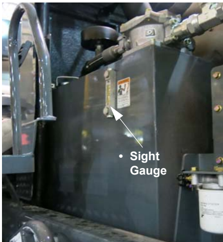
Hydraulic Oil Reservoir (Located on left-hand side of machine - open hood to access) -Typical View
