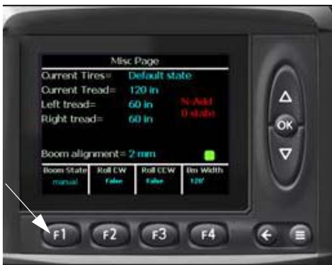
F1 Switch - Boom State (Located on the MD3 Monitor - Misc Page) -Typical View
