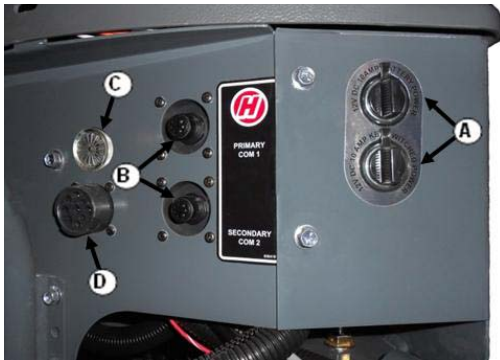
Electrical Ports (Located on back side of the side console) -Typical View
