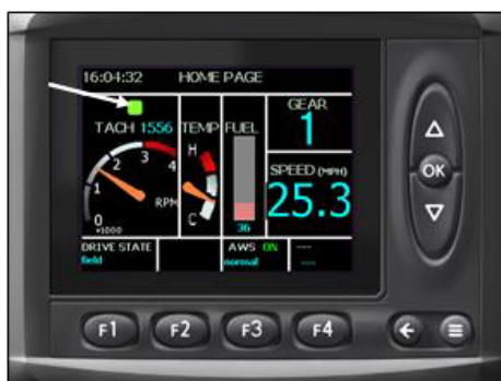
Main Spray Indicator (Located on the Home Page) -Typical View
