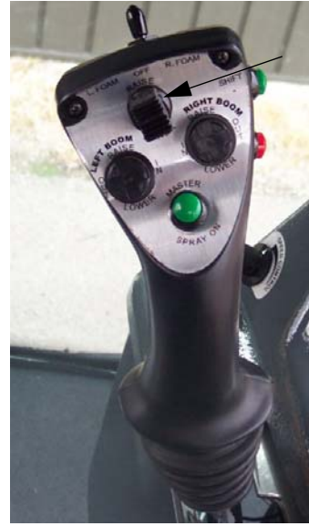
Transom Raise Switch (Located on the Hydrostatic Drive Control Handle) -Typical View
