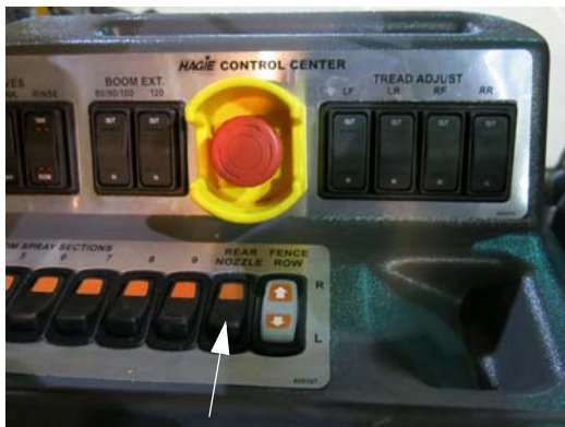
Rear Nozzle Switch (Located on the side console) -Typical View
