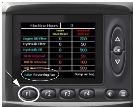
F1 (Reversible Fan) Button (Located on the MD3 Monitor) -Typical View
