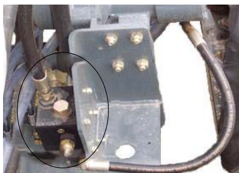
Pulse Width Modulated Control Valve -Typical View
