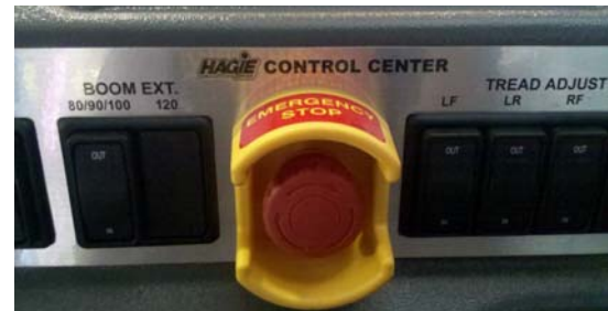
E-Stop Switch (Located on the side console) -Typical View
