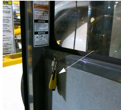
Emergency Exit Tool (Located on the right rear cab frame) -Typical View
