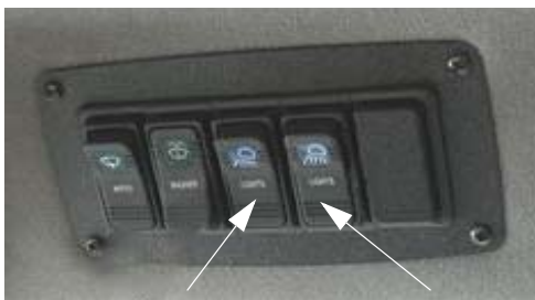
• Field Lights Switch • Work Lights Switch
