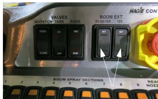
Boom Extension Switches (Located on the side console) -Typical View
