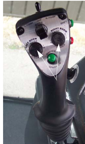
Left and Right Boom Switches (Located on the Hydrostatic Drive Control Handle) -Typical View
