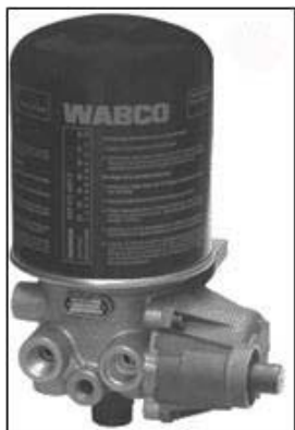
Air Dryer (Located beneath right-hand side of machine) -Typical View
