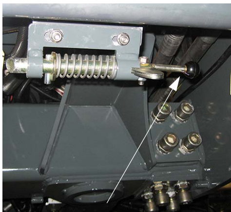
Front Fill Release Lever (Located beneath front end of machine) -Typical View
