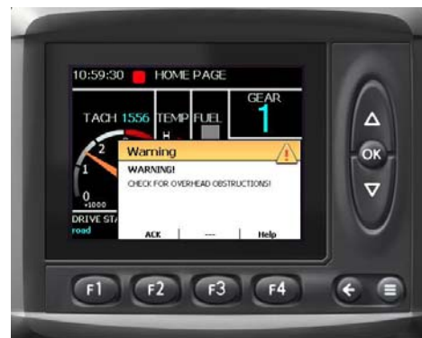
Power Line Warning Message (Located on the MD3 Monitor) -Typical View
