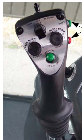
Speed Range Switches (Located on the side of the Hydrostatic Drive Control Handle) -Typical View
