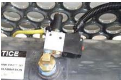
Pilot Valve (Located beneath catwalk on left-hand side of machine) -Typical View
