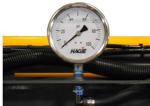
Pressure Gauge -Typical View
