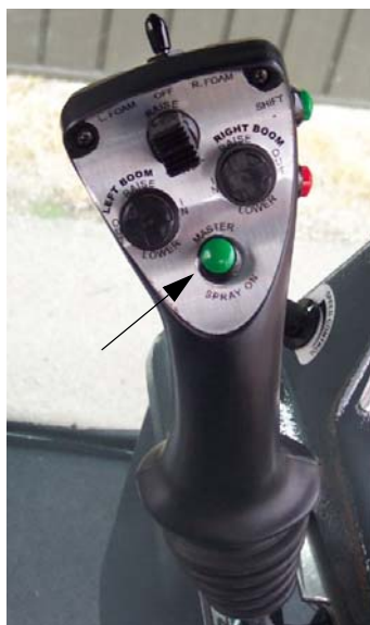
Master Spray Switch (Located on the Hydrostatic Drive Control Handle) -Typical View
