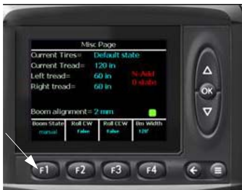
F1 Switch - Boom State (Located on the MD3 Monitor - Misc Page) -Typical View
