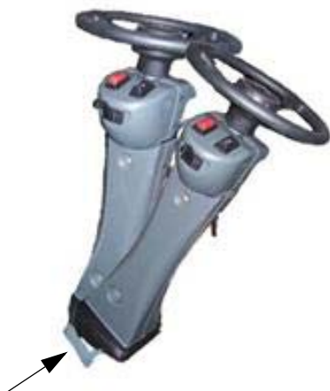
Steering Column Release Pedal (Located on the lower left-hand side of steering column) -Typical View
