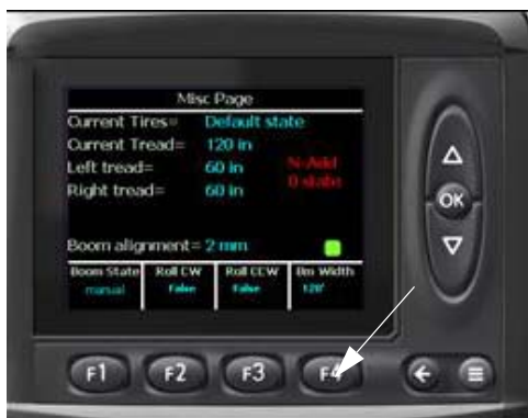
F4 Switch - Spray Width (Located on the MD3 Monitor - Misc Page) -Typical View
