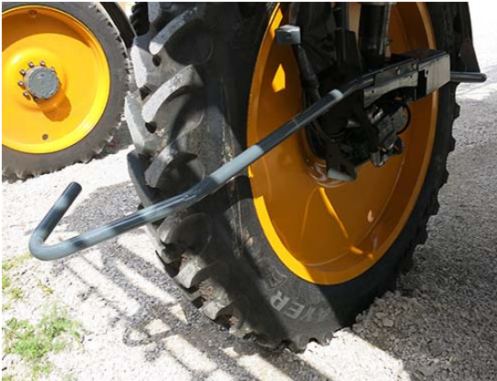
Installed Crop Divider -Typical View
