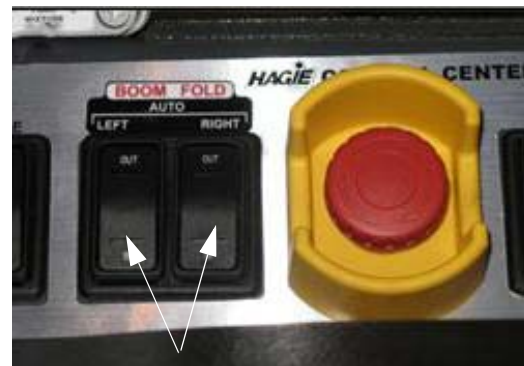
Auto Fold Switches (Located on the side console) -Typical View
