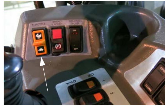
Throttle Switch (Located on the side console) -Typical View
