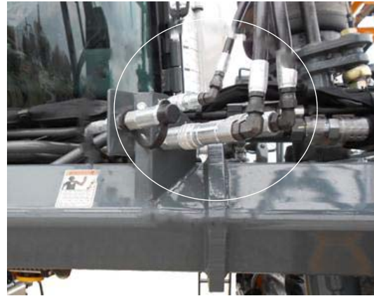
Hydraulic Connections (Located on front left-hand side of machine) -Typical View
