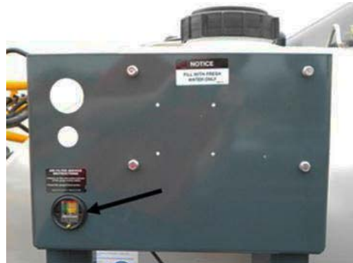
Filter Minder (Located on the Foam Marker tank mounting bracket) -Typical View
