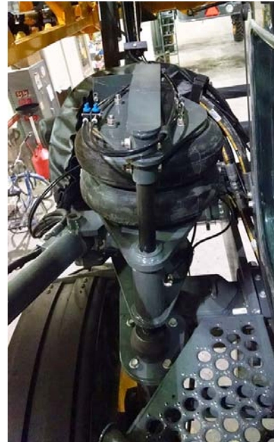
Air Bag (Located on each leg) -Typical View * Front Air Bag Shown
