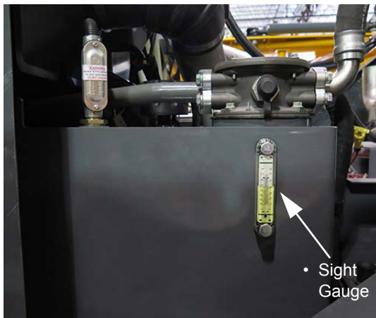
Hydraulic Oil Reservoir (Located on left-hand side of machine - open hood to access) -Typical View
