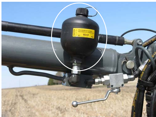
Accumulator -Typical View
