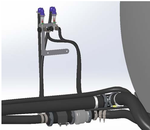
Flow Indicators (Located on the exterior right-hand side of cab) -Typical View * 2-pump configuration shown
