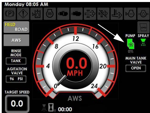
Solution Pump Indicator (Located on the Machine Display Home Page - Field Mode)
