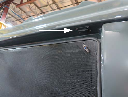
Hood Switch (Located ahead of rear hood above the radiator screen) -Typical View
