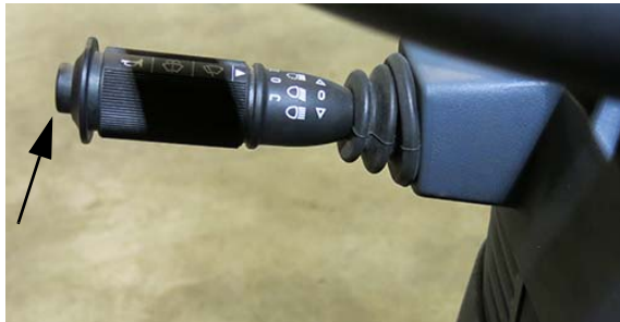
Horn Button (Located on the end of the turn signal lever) -Typical View
