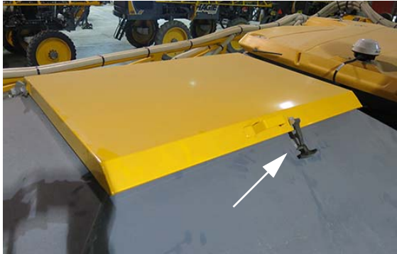
Security Latch (Located along side of the dry box lid) -Typical View
