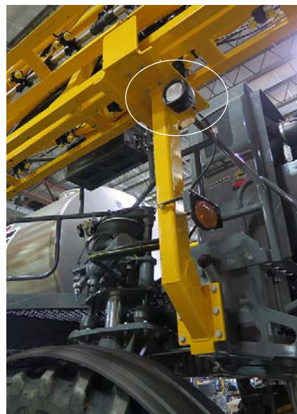
Work Lights (2) (Located on each boom cradle) -Typical View
