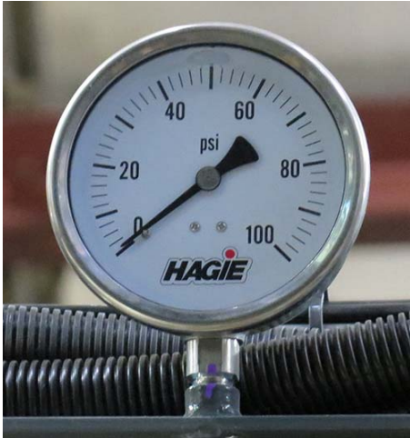
Pressure Gauge (Mounted on boom) -Typical View
