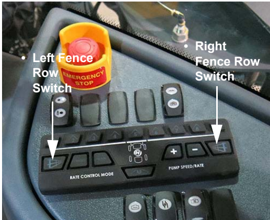
Left Fence Row Switch Right Fence Row Switch Fence Row Switches - Left and Right (Located on the side console) -Typical View
