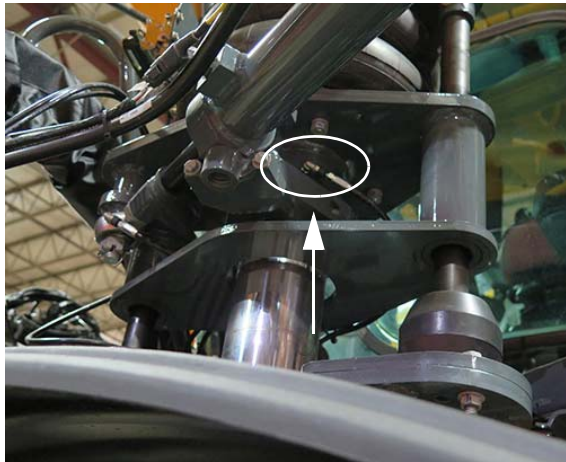
Collar Grease Zerk (4) (Located beneath each air bag mounting plate) -Typical View
