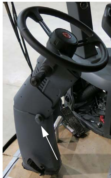
Steering Column Tilt Adjust Button (Located on the left-hand side of the steering column) -Typical View
