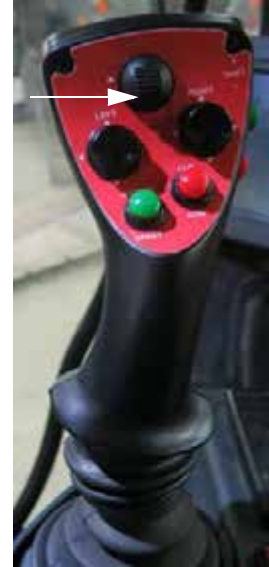
Transom Switch - DOWN (Located on the Hydrostatic Drive Control Handle) -Typical View
