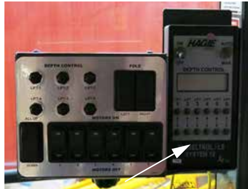
Tasselrol Control Panel -Typical View
