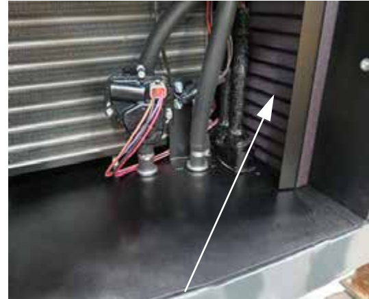
Recirculation Filter (Located along the right-hand side of compartment) -Typical View
