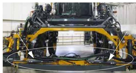
Main Pivot/Breakaway Cylinders -Typical View
