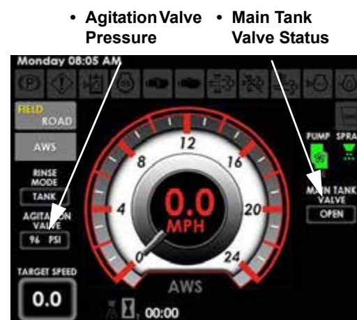
Main Tank Valve Status and Agitation Valve Pressure Indicators (Located on the Machine Display Home Page - Field Mode)
