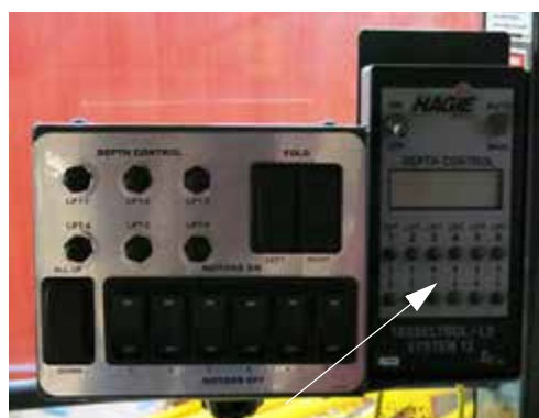
Tasselrol/LS System 12 Control Panel -Typical View
