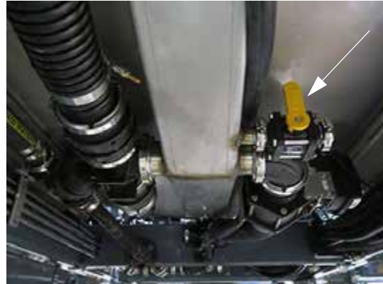
Solution Tank Drain Valve (Located beneath the solution tank on underside of machine) -Typical View
