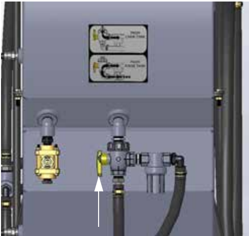
Inlet Selector Valve - 60 Gallon/227 L Tanks (Located on the outer side of Tanks 1 and 3) -Typical View * 3-Injection Pump Configuration
