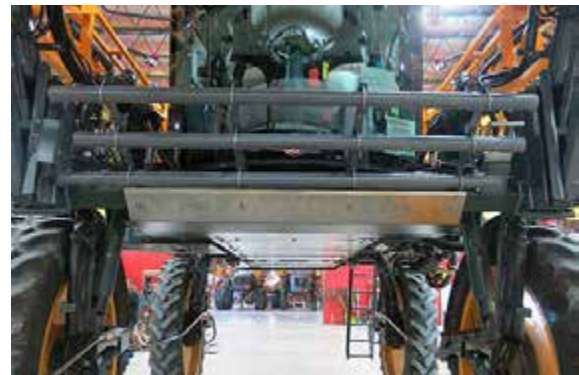
Brush Guard Installation -Typical View
