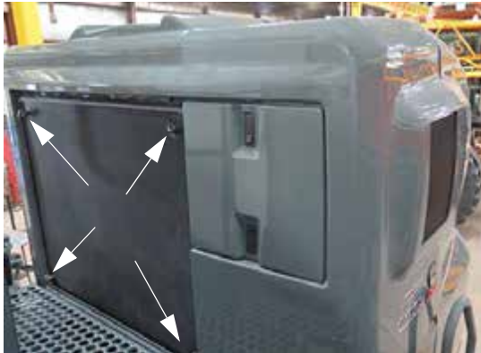
Radiator Screen Latches (Located on each corner of the screen) -Typical View
