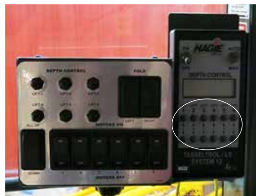
Lift Up/Down Switches (Located on the Tasseltról Control Panel) -Typical View
