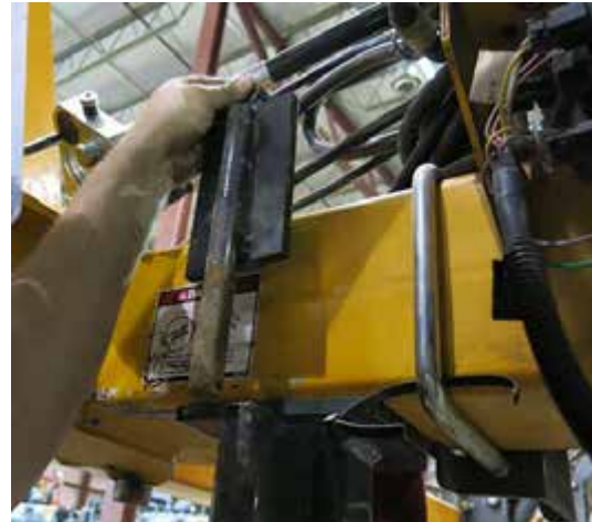
Stop Plate (Located on the inward side of each combo attachment stand) -Typical View
