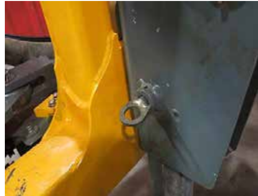
Lock Pin Removed -Typical View
