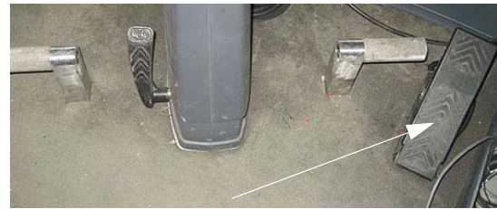
Decel Pedal (Located on the lower right-hand side of the steering column) -Typical View
