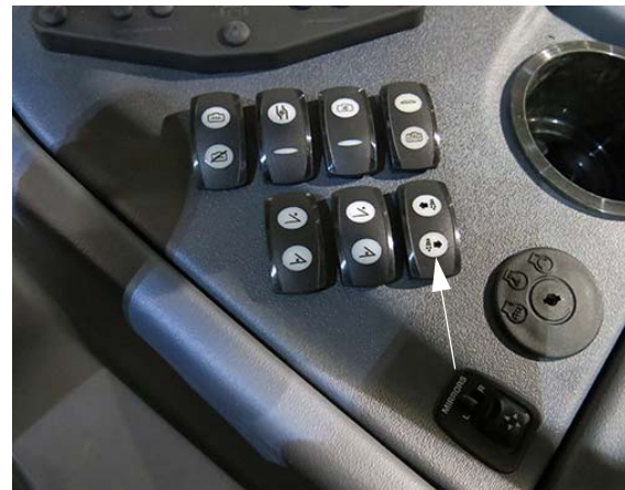
Foam Marker Switch (Located on the side console) -Typical View
