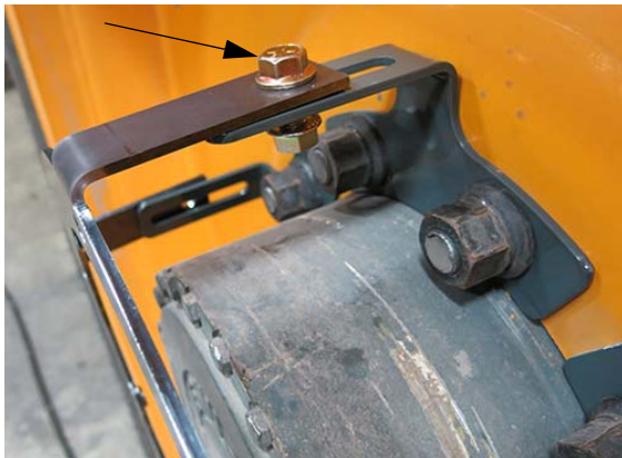
Hub Cap Adapter Bolt Installation -Typical View
