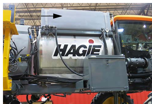
Rinse Tank -Typical View
