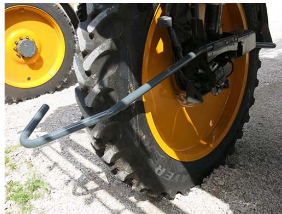
Installed Crop Divider -Typical View
