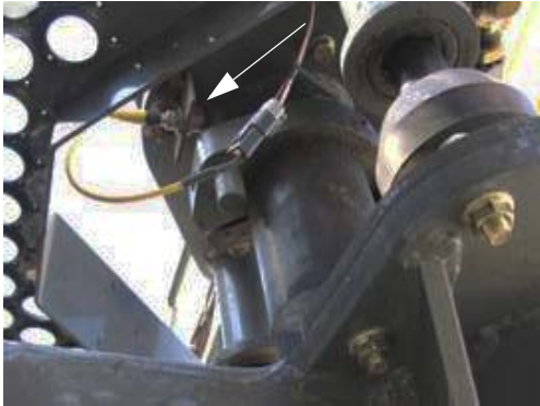
External Proximity Sensor -Typical View
