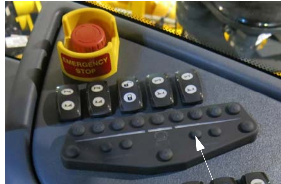
“+” Pump Speed/Rate Switch (Located on the side console) -Typical View
