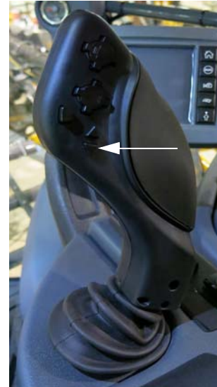
Transom Switch - DOWN (Located on the Hydrostatic Drive Control Handle) -Typical View
