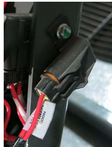
Hood Actuator Fuse (Located near rear left-hand side of machine - open hood to access) -Typical View
