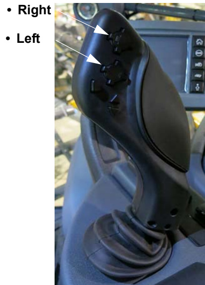
Left and Right Boom Switches (Located on the Hydrostatic Drive Control Handle) -Typical View
