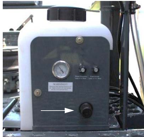
Foam Pressure Dial (Located on the side of the Foam Marker Tank) -Typical View
