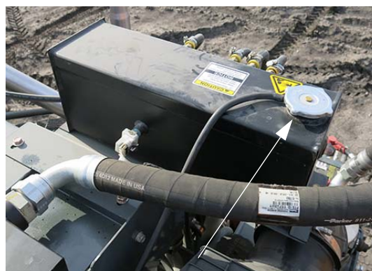
Radiator Cap (Located in the engine compartment) -Typical View
