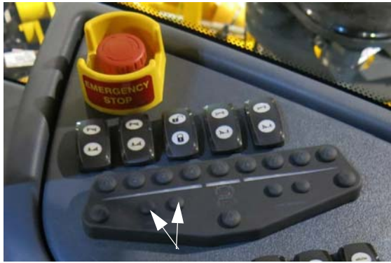
Rate Control Switches (Located on the side console) -Typical View
