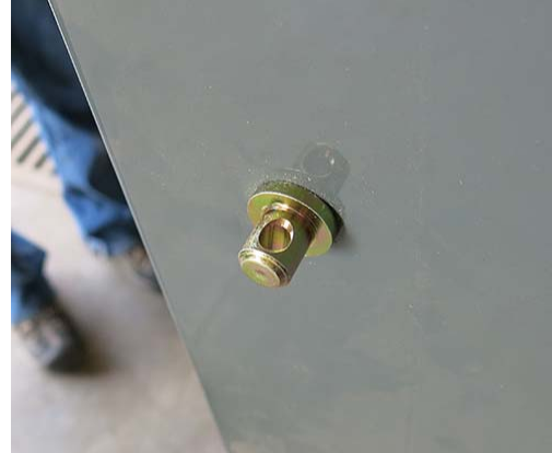
Hanger Pin Installation -Typical View
