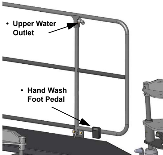
Upper Water Outlet/Hand Wash Foot Pedal (Mounted on left-hand handrail near cab door) -Typical View
