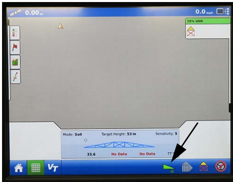
Auto/Manual Button - Ag Leader (Located on the main “Run Screen”) -Typical View
