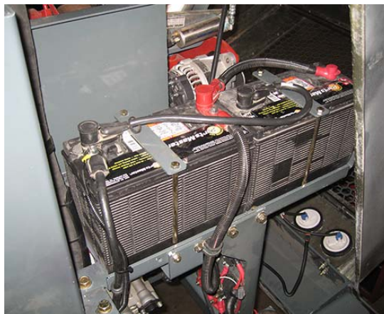
Battery Access (Located on the rear left-hand side of machine - open hood to access) -Typical View
