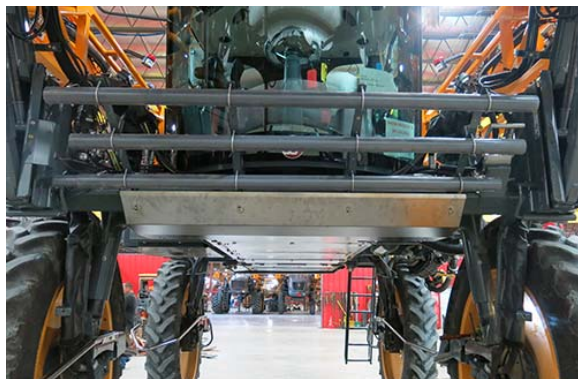
Brush Guard Installation -Typical View
