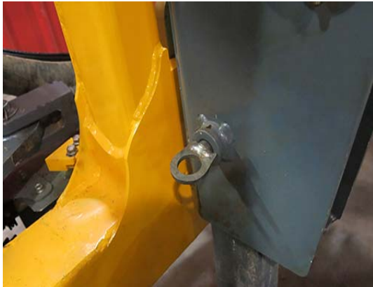
Lock Pin Removed -Typical View
