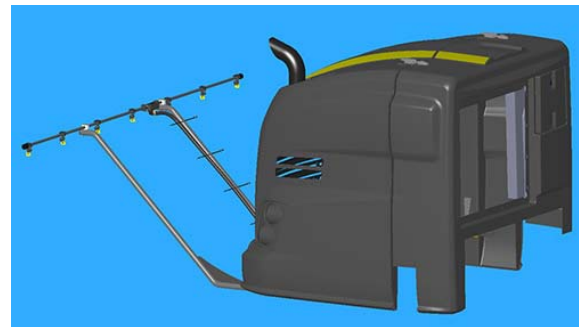
Rear Boom Installation -Typical View
