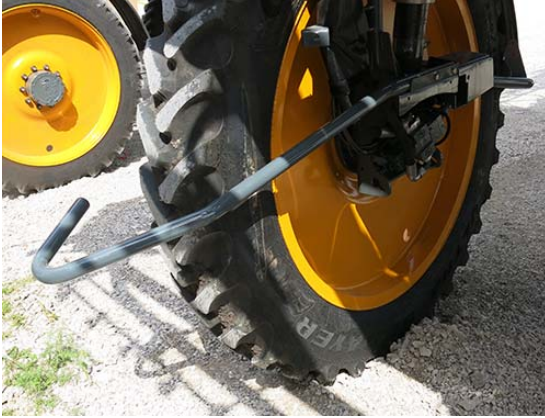
Installed Crop Divider -Typical View
