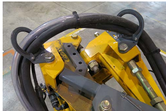
Boom Hose Clamp Installation -Typical View
