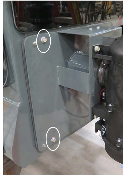
Mounting Bolts (4) (Two located on each side of access panel on the right-hand side of cab) -Typical View
