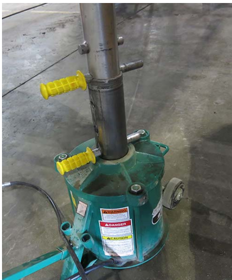
Lock Pin Installation -Typical View
