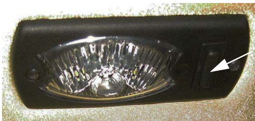
Interior Work Light Switch -Typical View
