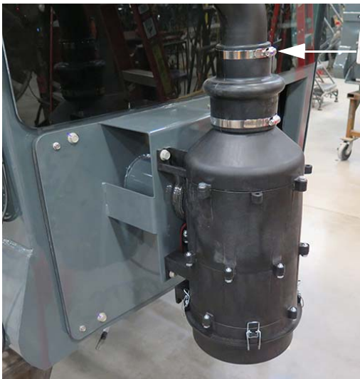
Flange Clamp - Top (Located near the top of the RESPA filtration unit) -Typical View
