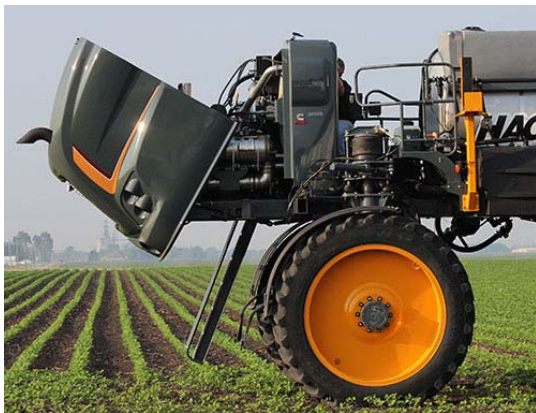
Rear Hood (Open position shown) -Typical View
