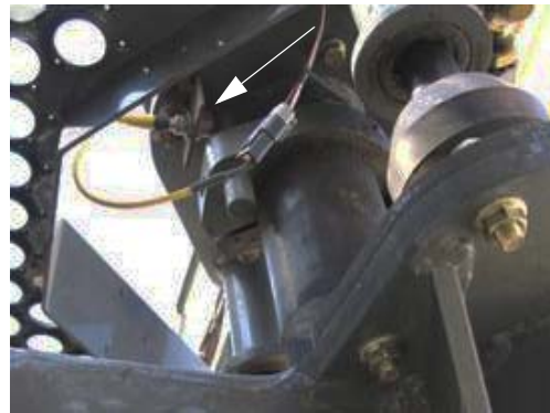
External Proximity Sensor -Typical View
