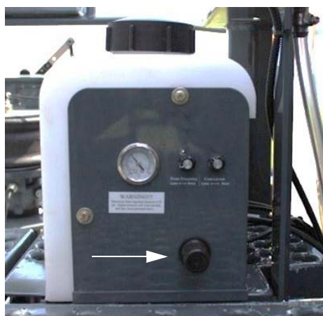
Foam Pressure Dial (Located on the side of the Foam Marker Tank) -Typical View
