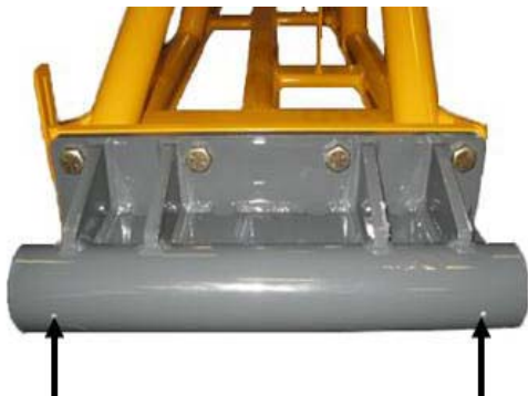
Boom Adapter -Typical View
