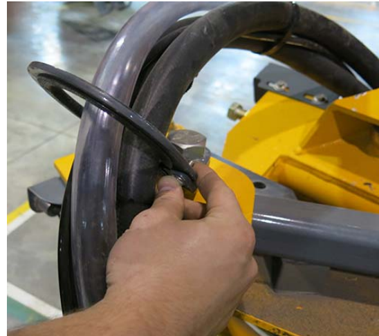
Boom Hose Clamp -Typical View
