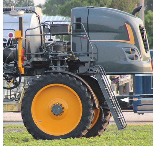
Ladder -Typical View * Lowered position shown
