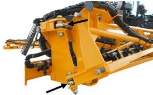
Boom Fold Linkages -Typical View
