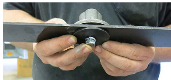
Cutter Blade Assembly -Typical View
