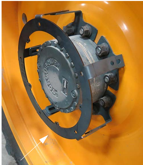
Hub Cap Adapter Weldment -Typical View
