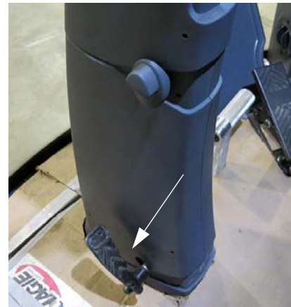
Steering Column Release Pedal (Located on the lower left-hand side of the steering column) -Typical View
