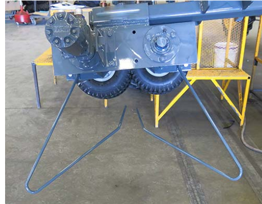
Stalk Guide Installation -Typical View
