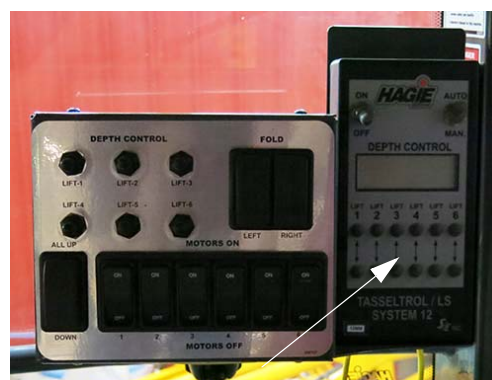
Tasseltrol/LS System 12 Control Panel -Typical View
