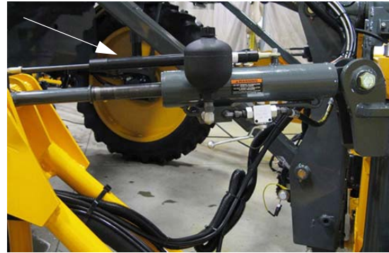
Position Sensor -Typical View
