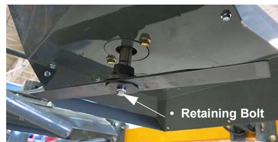
Cutter Blade Assembly (Mounted on the bottom side of Cutter Head) -Typical View
