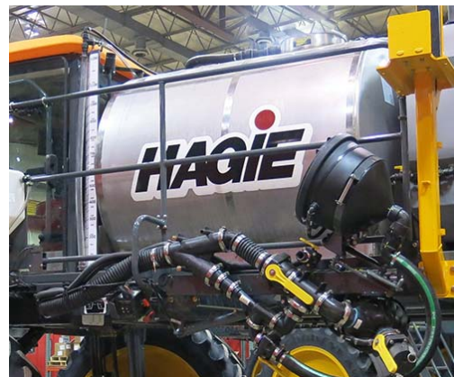
Solution Tank -Typical View
