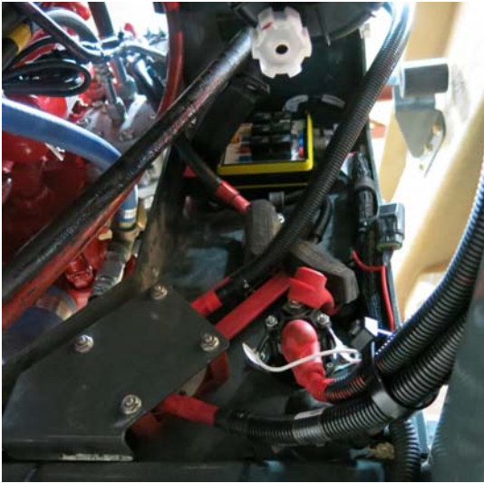
Tier 4 Final Engine Fuse/Relay Block (Located beneath batteries on the rear left-hand side of machine)
