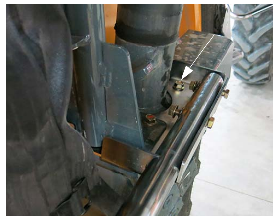
Mounting Plate Bolt -Typical View
