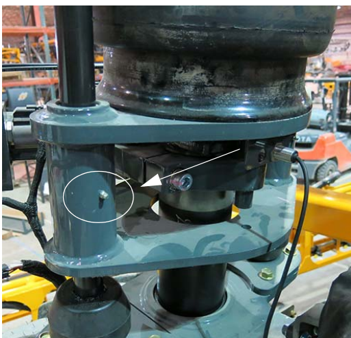
Tower Bearing Grease Zerk (Located on the front and rear legs) -Typical View
