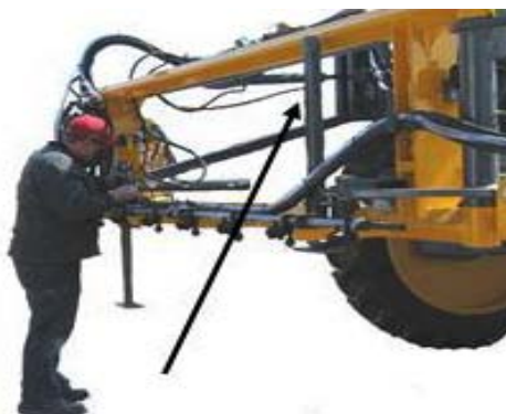
Boom Stand in “Travel” Position -Typical View
