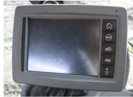
Machine Display -Typical View
