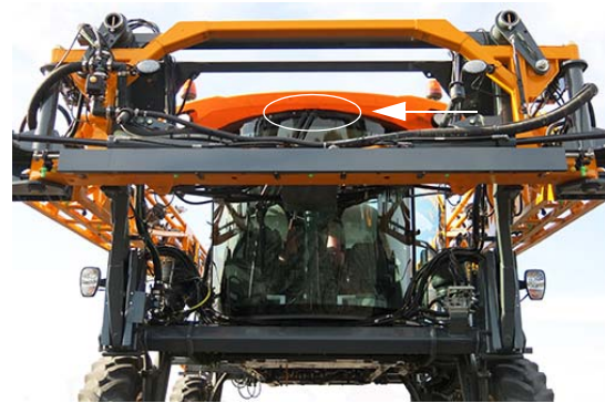
Windshield Washer Fluid Spray Nozzle (Located near top of exterior cab) -Typical View
