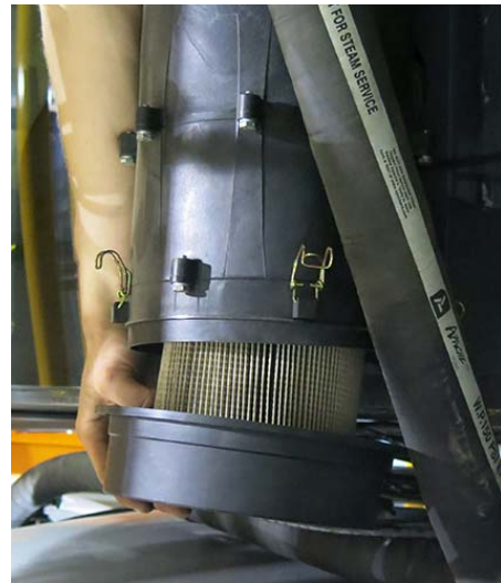
Filter Removal -Typical View
