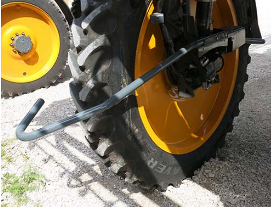
Installed Crop Divider -Typical View
