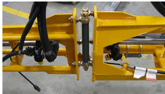
Outer Breakaway -Typical View
