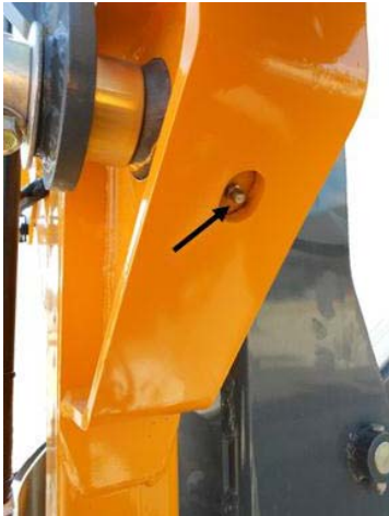
Pivot Transom Ball Joints -Typical View
