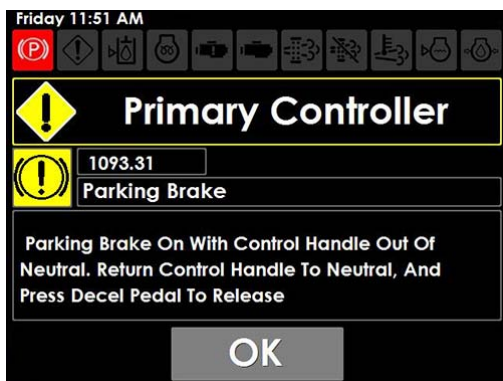
Parking Brake Warning Message
