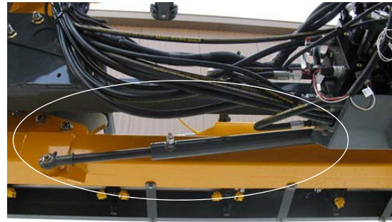
Roll Cylinder -Typical View
