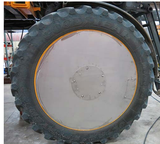
Wheel Cover Installation -Typical View
