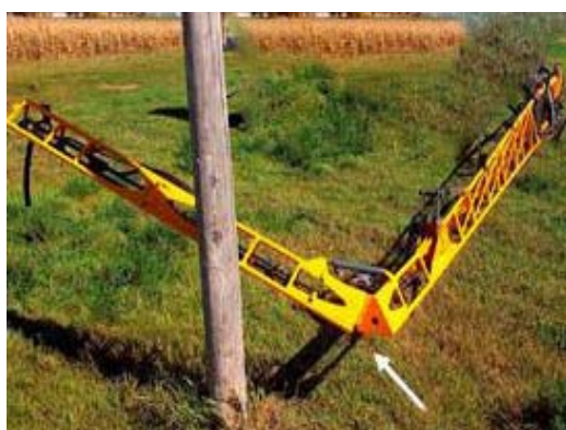
Outer Boom Breakaway -Typical View
