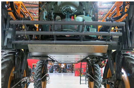
Brush Guard Installation -Typical View
