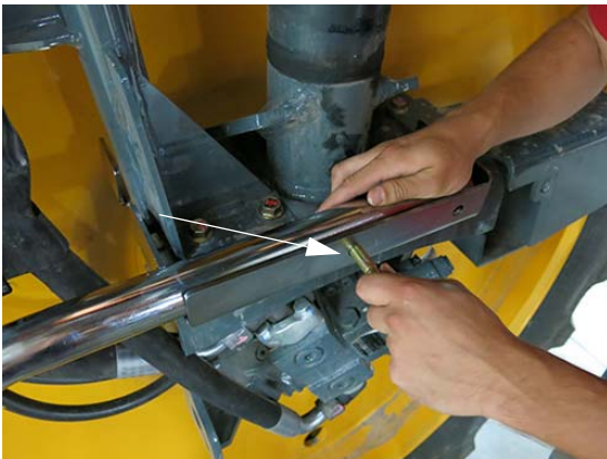
Crop Divider Mounting Bolt -Typical View
