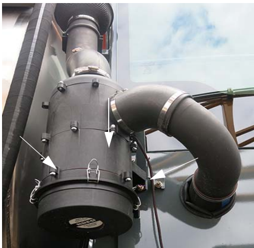
Filter Latches -Typical View
