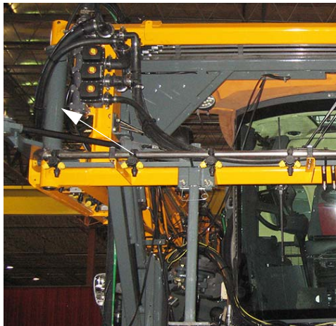
Transom Pivot Tube -Typical View
