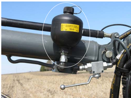
Accumulator -Typical View
