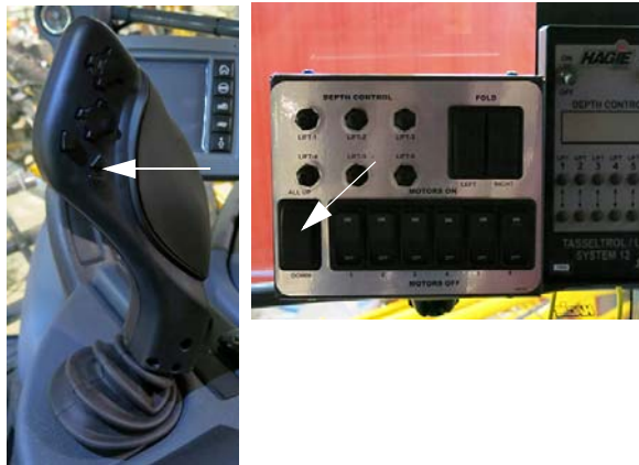
All-Up/Down Switch (Located on the Hydrostatic Drive Control Handle or the Detasseling Control Panel) -Typical View
