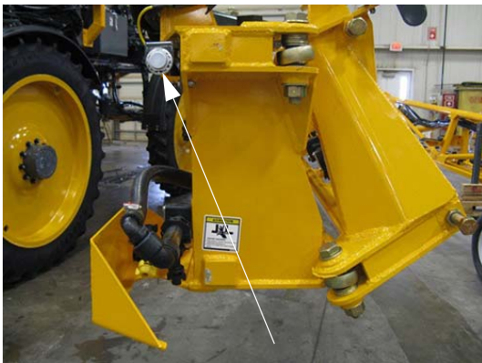
Proximity Sensors -Typical View
