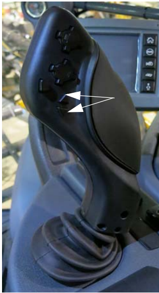
Transom Switches (Located on the Hydrostatic Drive Control Handle) -Typical View
