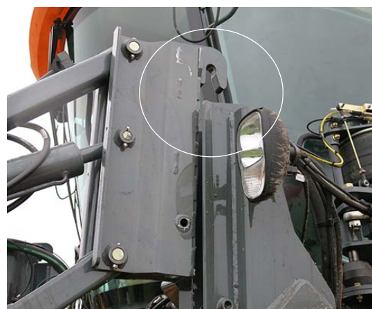
Attachment Clearing Mounting Pin -Typical View
