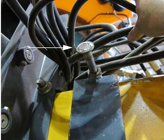
Securement Pin (Located on the inward side of each combo attachment stand) -Typical View
