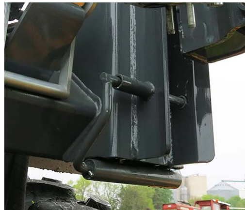
Lock Pin -Typical View * Engaged position shown
