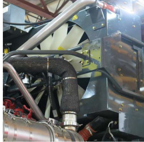
Reversible Fan (Located near rear of machine - open hood to access) -Typical View
