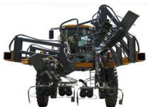
Staggered Detasseling Heads -Typical View
