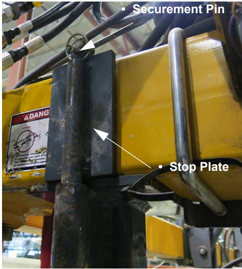
Stop Plate/Securement Pin Assembly -Typical View
