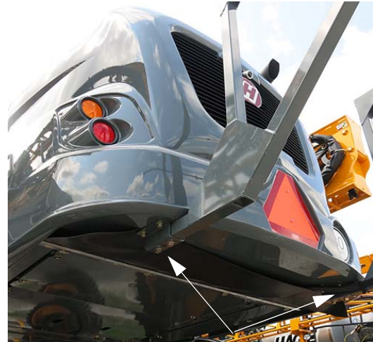
Brush Curtain Attached to Hood -Typical View
