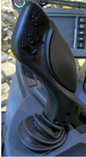
Hydrostatic Drive Control Handle -Typical View
