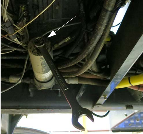
Pressure Filter Housing (Located beneath right-hand side of machine - lower metal shield to access) -Typical View
