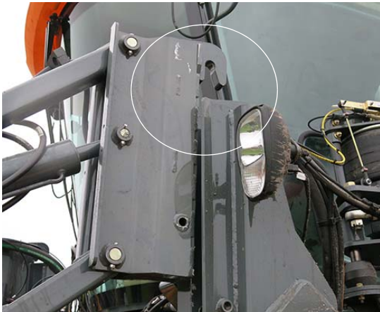
Attachment Clearing Mounting Pin -Typical View
