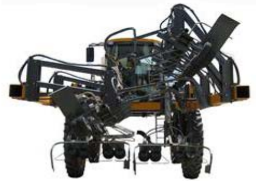
Staggered Detasseling Heads -Typical View
