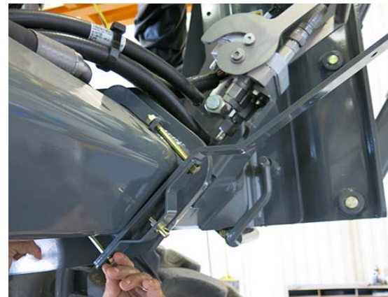
Anchor Bolt Assembly -Typical View
