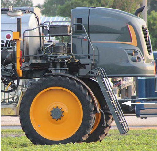
Ladder -Typical View * Lowered position shown
