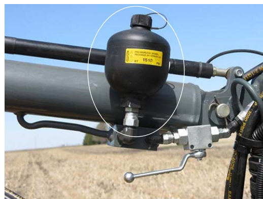
Accumulator -Typical View
