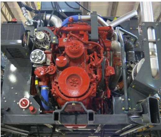
Tier 4 Diesel Engine -Typical View
