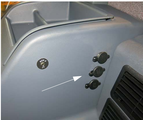
12V Power Ports -Typical installation shown
