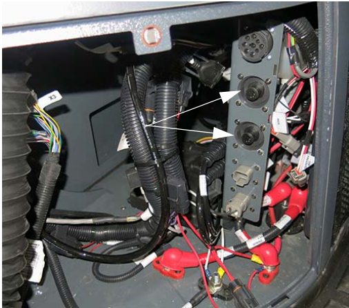
Hagie Diagnostic Ports (2) (Located inside the side console - remove front panel to access) -Typical View
