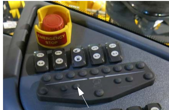
Manual “MAN” Rate Control Switch (Located on the side console) -Typical View
