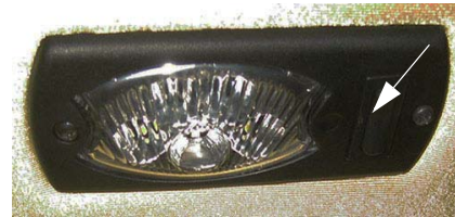
Interior Work Light Switch -Typical View
