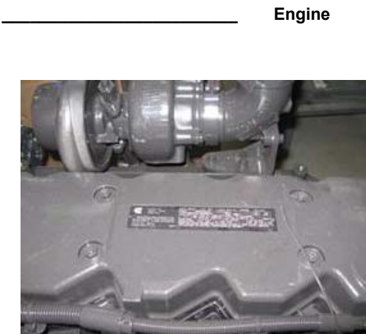
Engine Serial Number -Typical View
