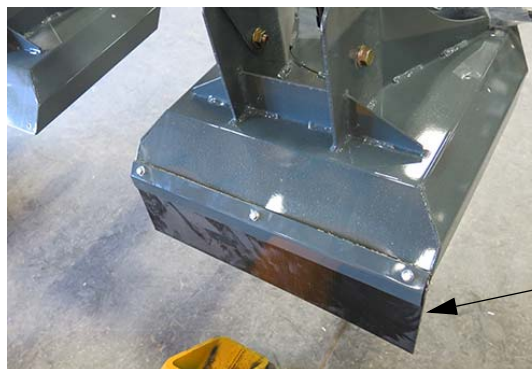
Cutter Head Extension Flap -Typical View
