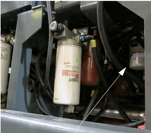
Engine Oil Filter (Located along left-hand side of machine) -Typical View
