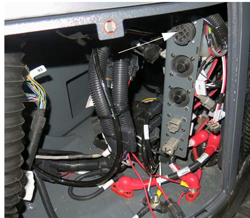
Engine Diagnostic Port (Located inside the side console - remove front panel to access) -Typical View
