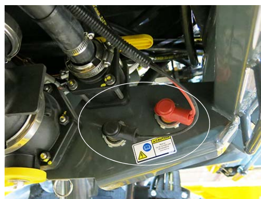
Power Ports (Located near front fill assembly) -Typical View
