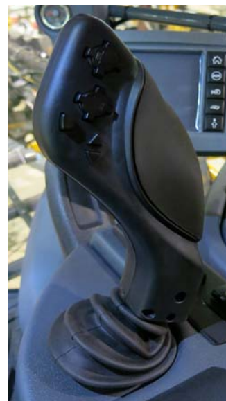
Hydrostatic Drive Control Handle (Located on the side console) -Typical View
