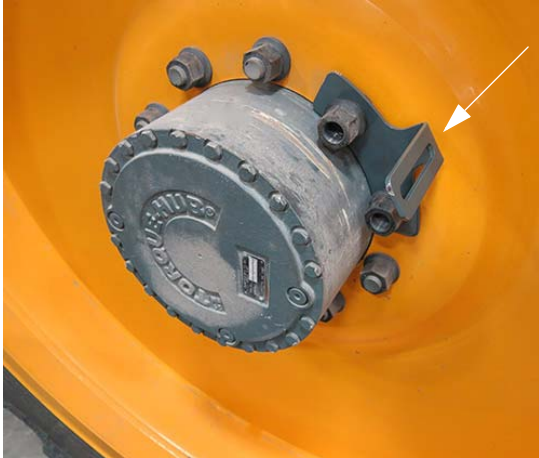
Hub Cap Adapter Plate -Typical View
