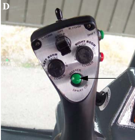
Master Spray Switch (Located on the Hydrostatic Drive Control Handle) -Typical View
