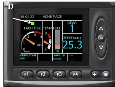
Float Indicator Light (Located on the MD3 Monitor) -Typical View
