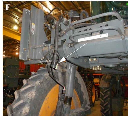
Electrical/Foamer Connections (Located on front right-hand side of machine) -Typical View
