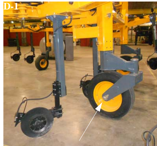
D-1 Gauge Wheel (One located on each side of NTB) -Typical View
