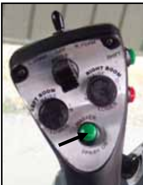
Figure 11: Master spray switch
