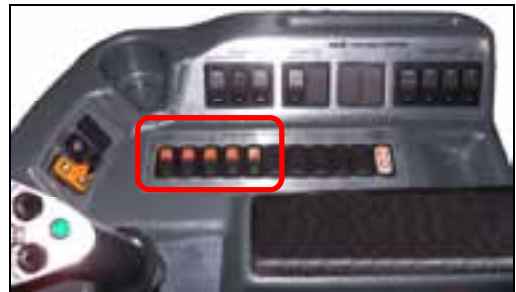
Figure 12: Spray section switches
