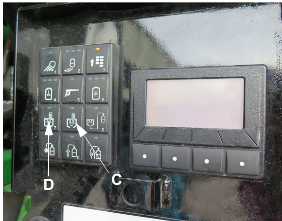
C - Eductor Rinse Button (filling from rinse tank) D - Eductor Rinse Button (filling from solution tank)
