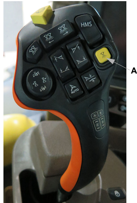
A - Spray System Master Switch
