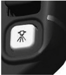
Spray System Master Switch
