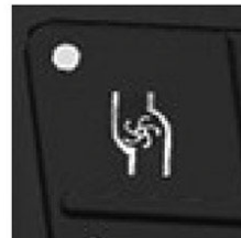
Solution Pump Switch
