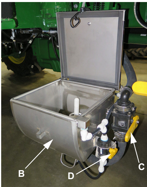
A - Educator Rinse Button B - Educator Tank (in working position) C - Rinse Valve D - Sump Valve
