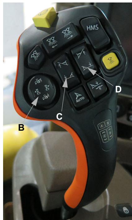
B - Center Boom Switch C - Left Boom Switch D - Right Boom Switch
