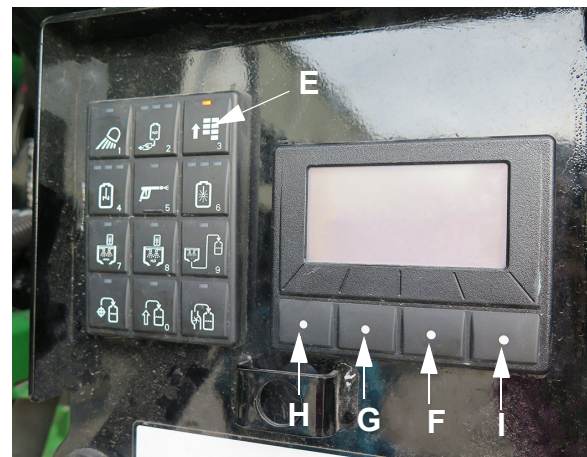
E - Rinse Tank Fill Button F - Auto Fill Button G - Manual Rinse Button H - Cancel Button I - Enter Button
