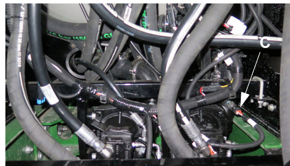
A - Flowmeter (2) B - Boom Pressure Sensor C - Solution Pump Pressure Sensor (2)
