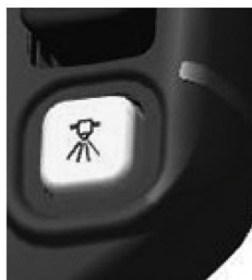
Spray System Master Switch
