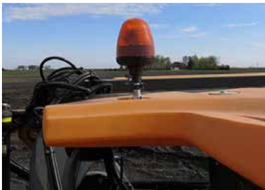
Rotating Beacon (2) (Located on each side of front roof cap) -Typical View
