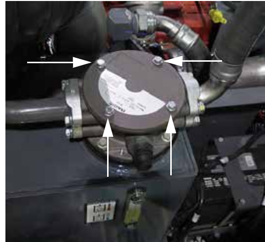
Return Filter Housing (Located on top of hydraulic oil reservoir) -Typical View
