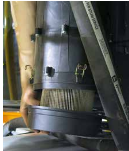
Filter Removal -Typical View
