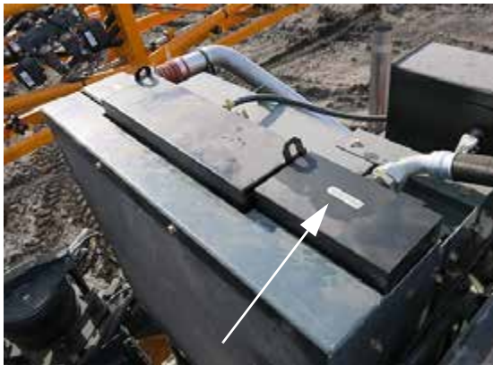
Oil Cooler (Located near rear of machine - open hood to access) -Typical View
