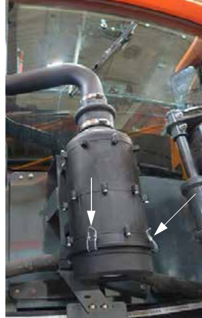
Filter Latches -Typical View
