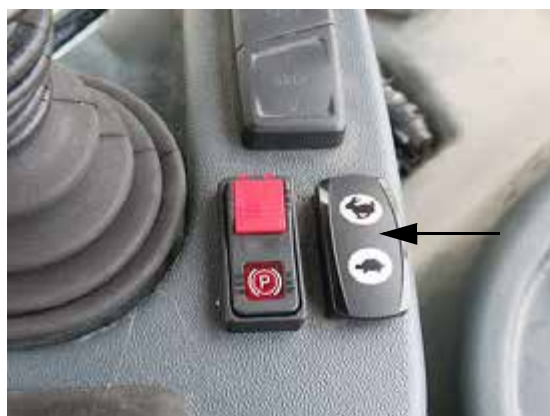
Throttle Switch (Located near the Hydrostatic Drive Control Handle) -Typical View
