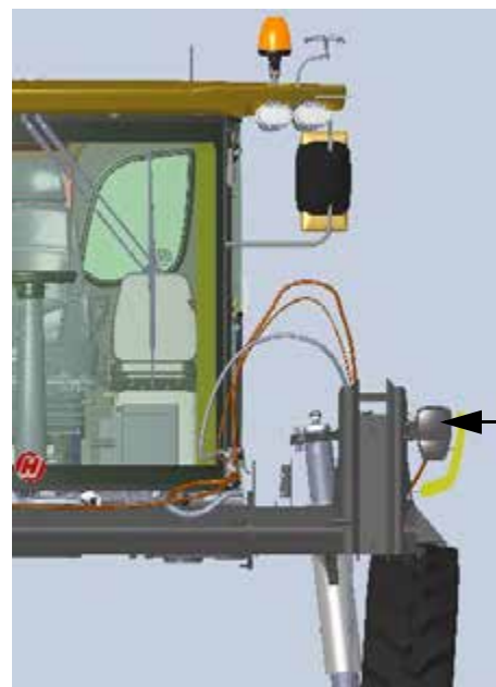
Highway Running Lights (2) -Typical View
