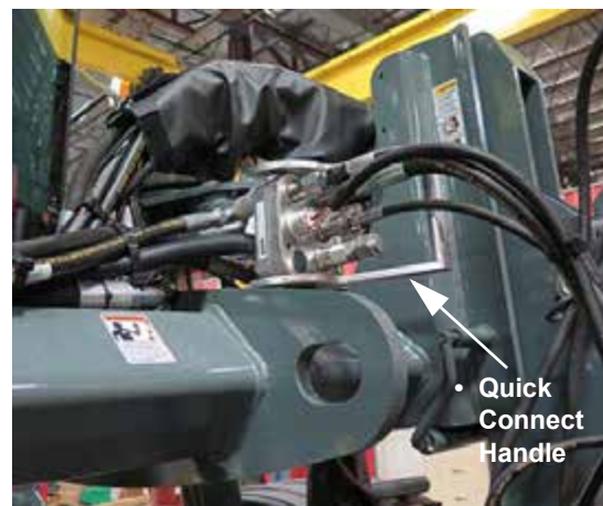
Hydraulic/Electrical Connections (Located on front left-hand side of machine) -Typical View * Push OUT to engage
