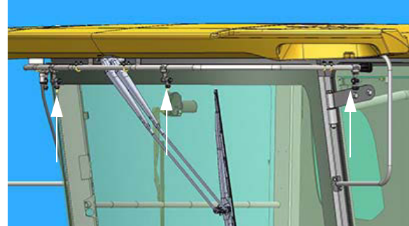
Deluge Spray Nozzles (Located around exterior cab) -Typical View
