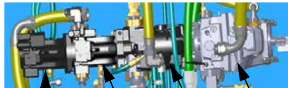
• PC Pump 1 • PC Pump 2 • LS Pump • Drive Pump
