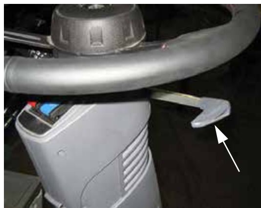
Steering Wheel Telescope Adjust Handle (Located on the right-hand side of steering column) -Typical View
