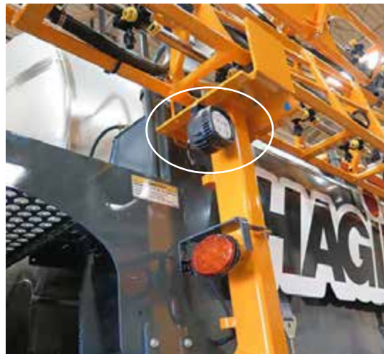
Work Lights (2) (Located on each boom cradle) -Typical View
