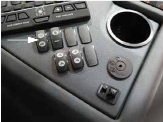
Main Tank Valve Switch (Located on the side console) -Typical View
