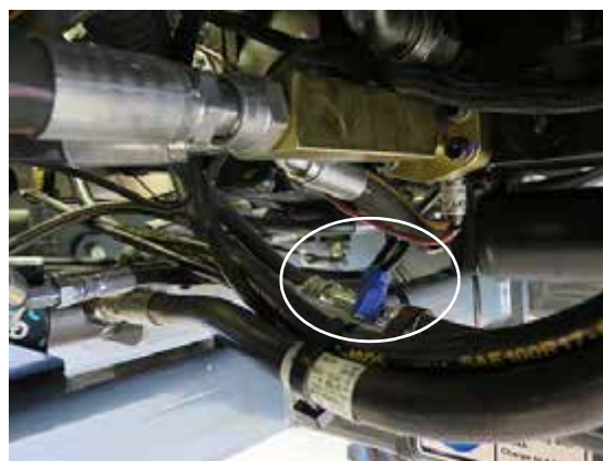
A/C Charge Ports (Located above mainframe on rear left-hand side of machine) -Typical View
