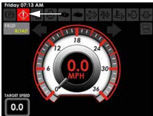
Warning Light Indicator (Located on the top left-hand side of each display page)
