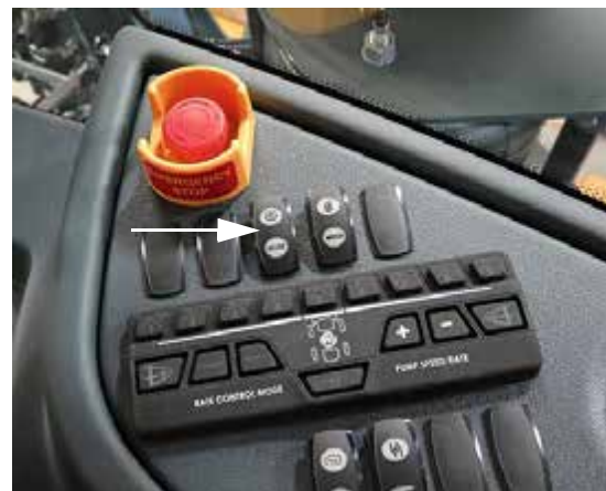
Deluge Switch (Located on the side console) -Typical View
