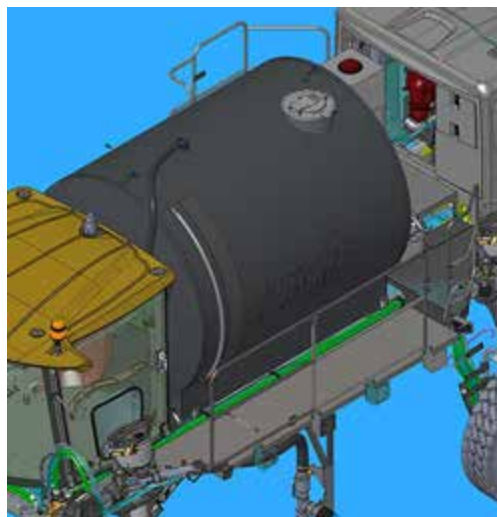
Solution Tank -Typical View
