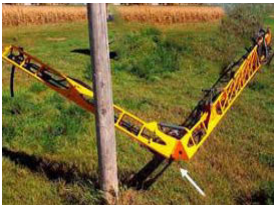
Outer Boom Breakaway -Typical View
