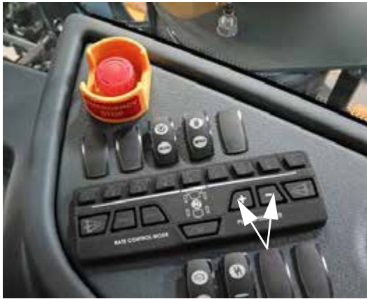
Pump Speed/Rate Switches (Located on the side console) -Typical View
