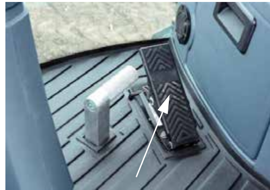
Decel Pedal (Located on the lower right-hand side of the steering column) -Typical View
