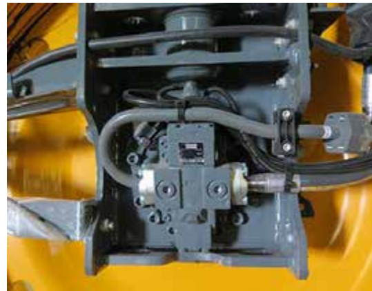
Wheel Motor -Typical View
