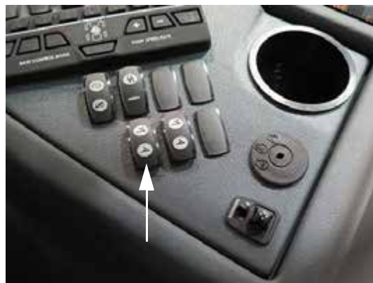
Boom Extension Switch (Located on the side console) -Typical View
