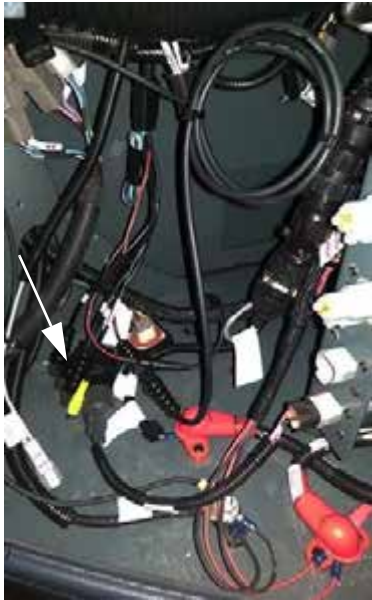
Belly Camera Input Connections (Located beneath side console - remove panel to access) -Typical View
