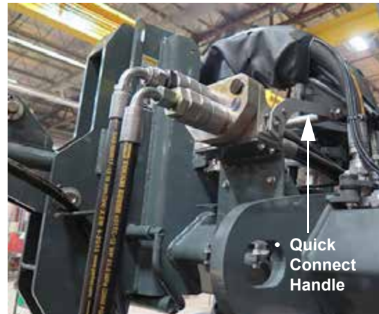
Hydraulic Connection (Located on front right-hand side of machine) -Typical View * Push UP to engage
