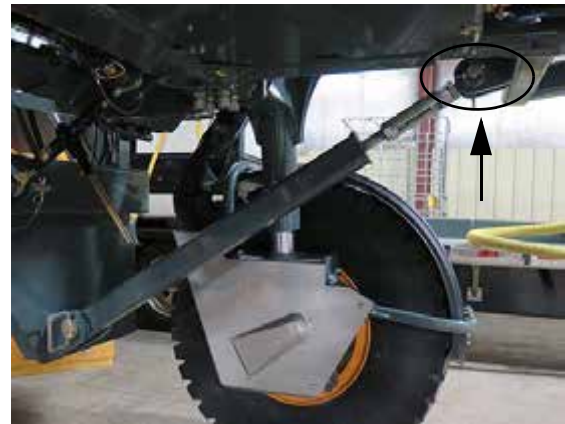
Securement Bolt/Nut Assembly - Upper -Typical View
