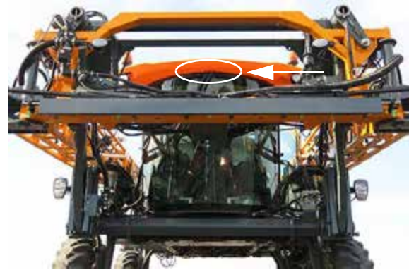
Windshield Washer Fluid Spray Nozzle (Located near top of front exterior cab) -Typical View
