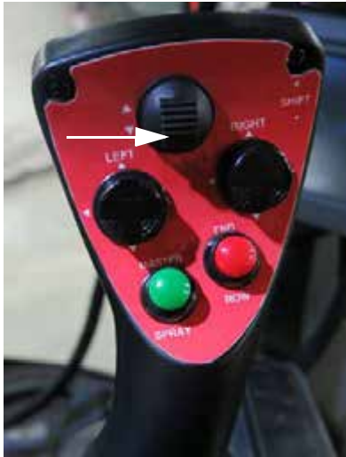
Transom Switch - DOWN (Located on the Hydrostatic Drive Control Handle) -Typical View
