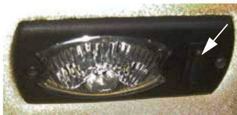
Interior Work Light Switch -Typical View
