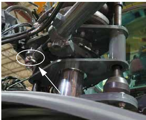
Tie Rod Ball Grease Zerk (2) (Located on the front legs) -Typical View
