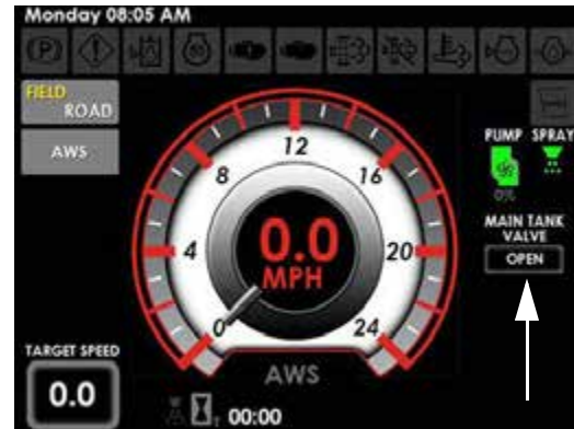
Main Tank Valve Status Indicator (Located on the Machine Display Home Page - Field Mode)
