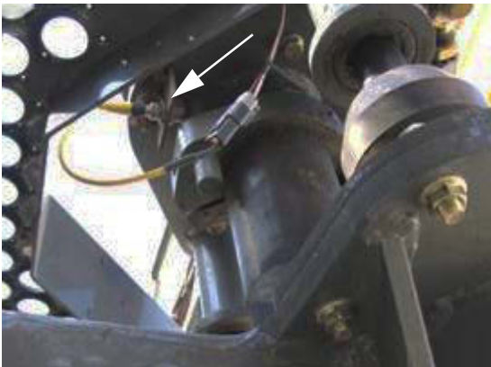
External Proximity Sensor -Typical View
