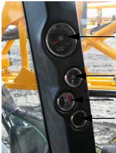
Machine Gauges (Located on cab A-post) -Typical View
