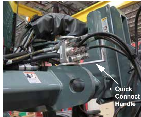
Hydraulic/Electrical Connections (Located on front left-hand side of machine) -Typical View * Push IN to disengage
