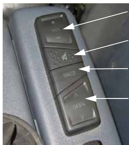
Remote Stereo Controls (Located near the Hydrostatic Drive Control Handle) -Typical View
