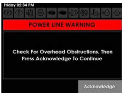
Power Line Warning Message (Located on the Machine Display)
