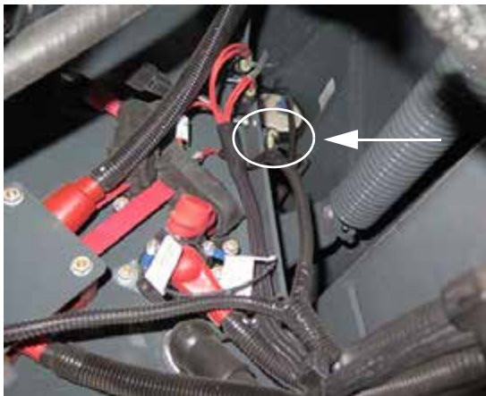
Hood Actuator Fuse (Located beneath rear left-hand side of machine) -Typical View
