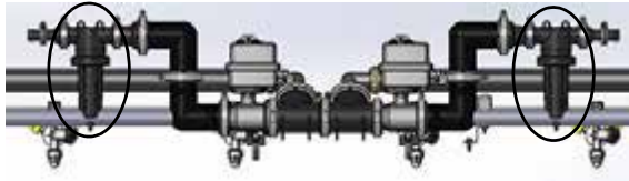
Section Strainers (Located throughout each boom section) -Typical View
