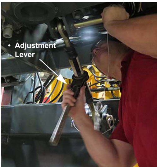
Top Link Arm Adjustment -Typical View
