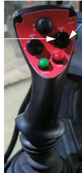
Plow Open/Close Switch (Located on the Hydrostatic Drive Control Handle) -Typical View
