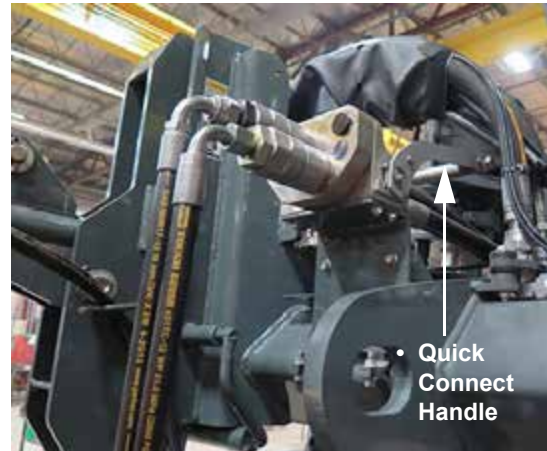
Hydraulic Connection (Located on front right-hand side of machine) -Typical View * Push DOWN to disengage
