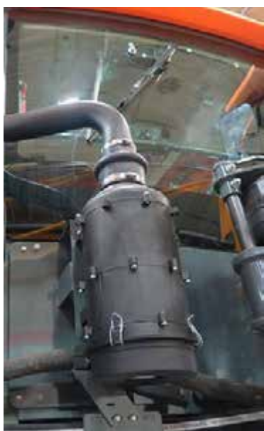
Cab Filtration System (Located on the right-hand side of the exterior cab) -Typical View
