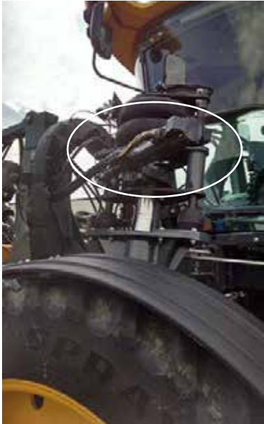
Steering Cylinder -Typical View
