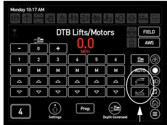
Lift Icon Buttons (All Up/Down) (Located on the Machine Display DTB Lifts/Motors Screen) -Typical View
