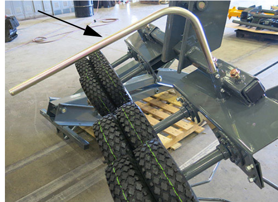
Deflector Shield Mounting Tube -Typical View
