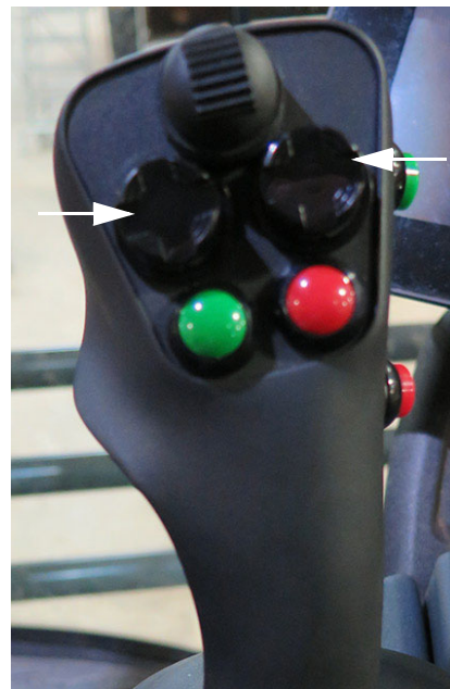
Outrigger Fold Switches - Left/Right (Located on the Hydrostatic Drive Control Handle) -Typical View
