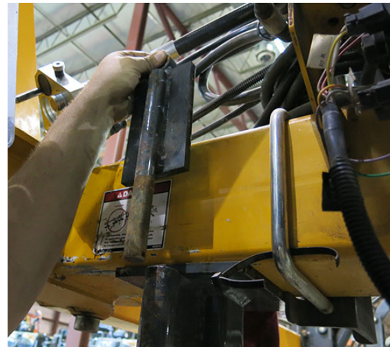
Stop Plate (Located on the inward side of each DTB attachment stand) -Typical View
