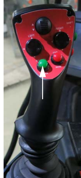
Main Control Switch (Located on the Hydrostatic Drive Control Handle) -Typical View
