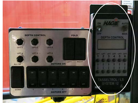
Tasseltrol/LS System 12 Control Panel -Typical View
