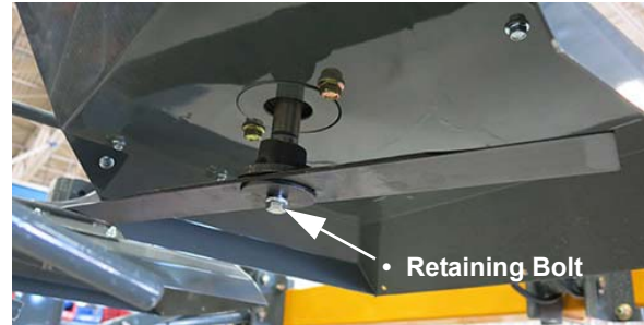
Cutter Blade Assembly (Mounted on the bottom side of Cutter Head) -Typical View
