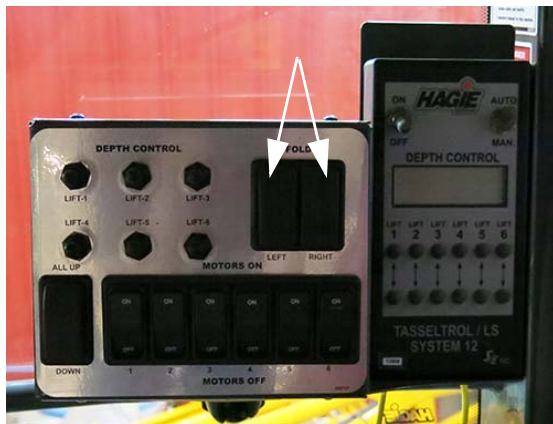
Outrigger Fold Switches - Left/Right (Located on the detasseling control panel) -Typical View
