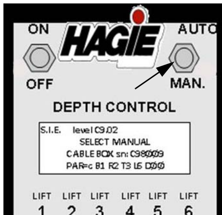
Auto/Manual Switch (Located on the Tasseltrrol/ LS System 12 Control Panel) -Typical View
