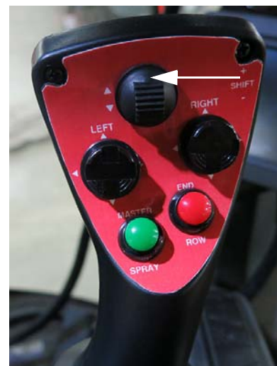
Transom Switch - UP (Located on the Hydrostatic Drive Control Handle) -Typical View
