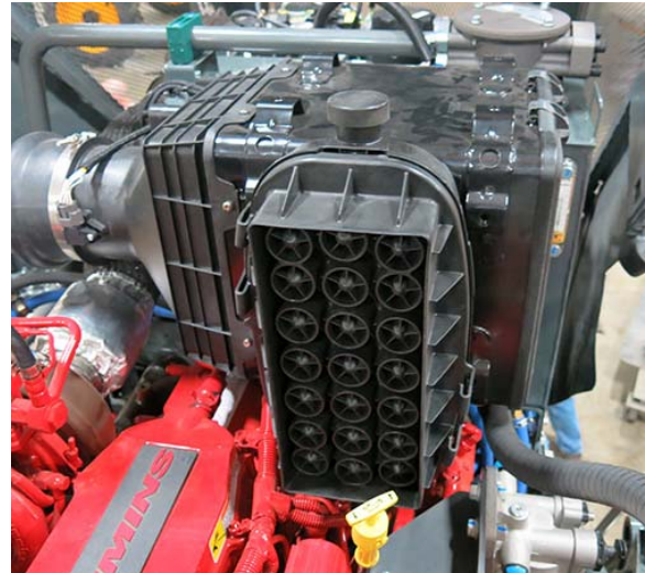
Engine Air Intake Filter (Located along platform on left-hand side of machine - open hood to access) -Typical View
