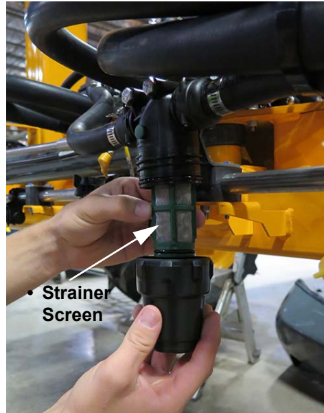
Section Strainer (Located throughout each boom section) -Typical View
