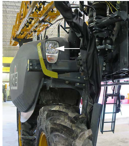
Highway Running Lights (2) -Typical View
