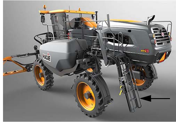
Ladder -Typical View * Lowered position shown
