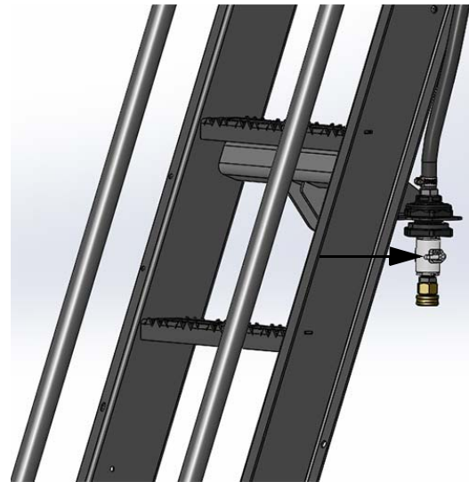
Hand Wash Valve (Ladder) -Typical View
