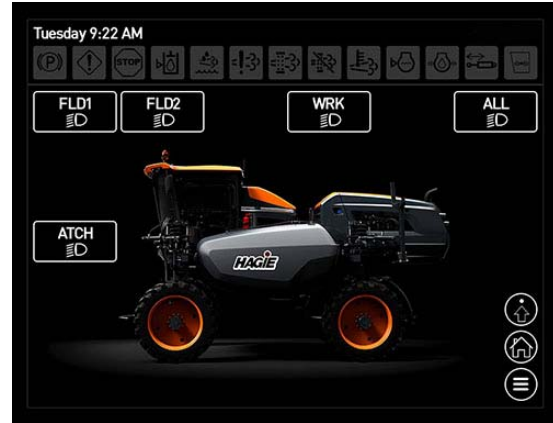
Exterior Lighting Screen
