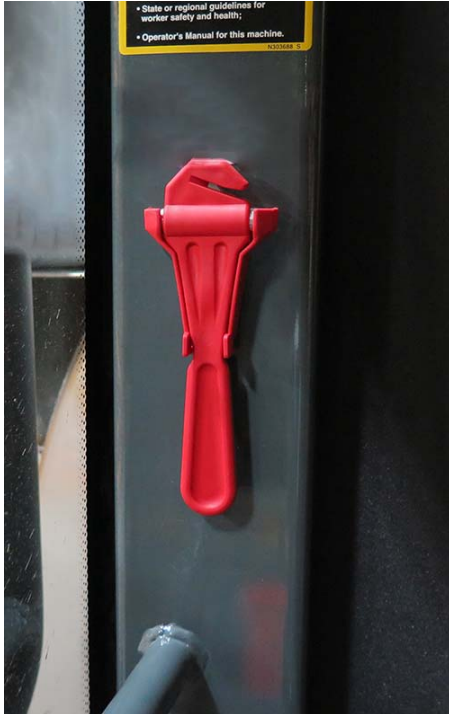
Emergency Exit Tool (Located along rear right-hand side of cab) -Typical View
