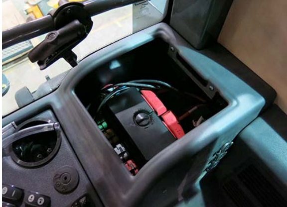
Circuit Breakers/Fuses (Interior) (Located rear of side console - remove tray to access) -Typical View
