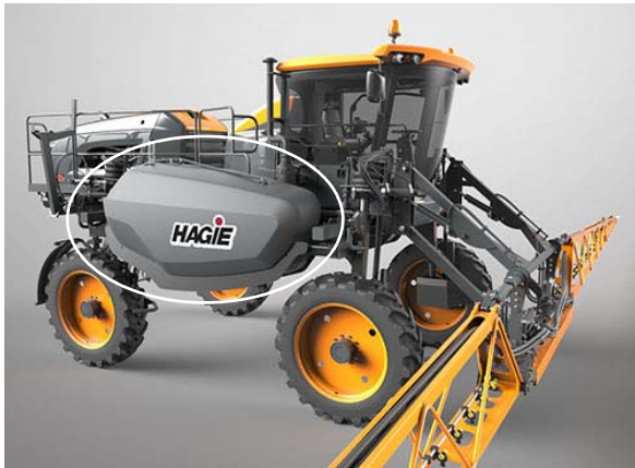
Solution Tank -Typical View
