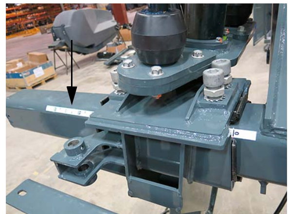
Tread Adjust Indicator (Located on slide path) -Typical View
