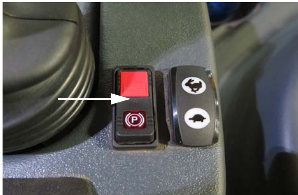
Parking Brake Switch (Located near the Hydrostatic Drive Control Handle) -Typical View
