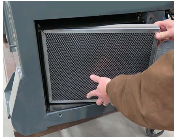
Charcoal Filter (Located behind the exterior service panel on the right-hand side of cab) -Typical View
