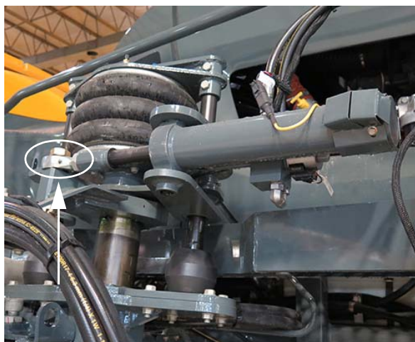
Tie Rod Ball Grease Zerk (Located on the front legs*) -Typical View
