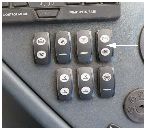
Agitation Valve Switch (Located on the side console) -Typical View
