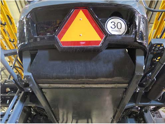
Brush Curtain Installation -Typical View
