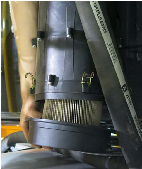
Filter Removal -Typical View
