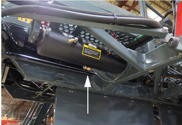
Tank Drain Valve (Main) (Located beneath platform on rear right-hand side of machine) * Pull DOWN to open -Typical View
