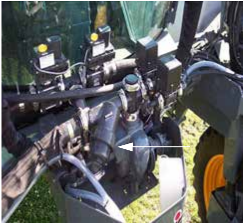
Solution Line Strainer (Located near front of machine behind the center front shield) -Typical View
