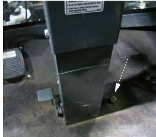
Master Spray Switch (Located on the lower right-hand side of steering column) -Typical View
