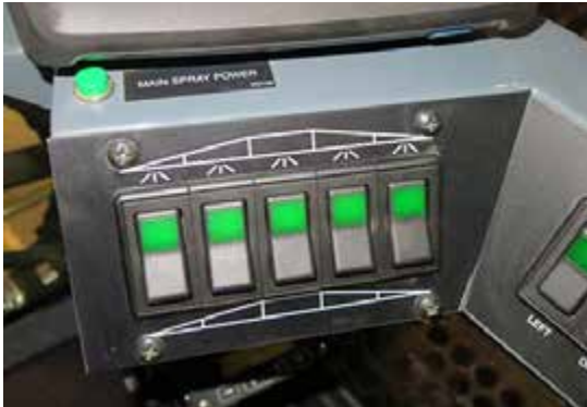
Boom Solution Valve Switches (Located on side console) -Typical View
