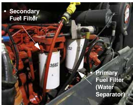
Primary and Secondary Fuel Filters (Located on left-hand side of engine - open hood to access) -Typical View
