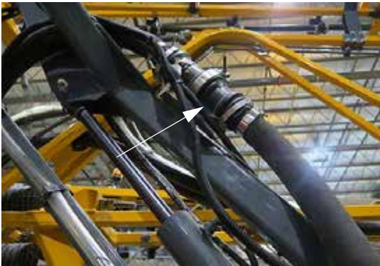
Flow Meter (Located on the right-hand side of machine) -Typical View
