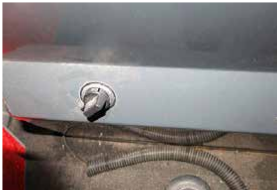
Power Port - Storage Console (Located on lower storage console on the left-hand side of operator's seat) -Typical View
