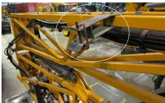
Lock Pin (Located near the rear of each folded boom extension) -Typical View
