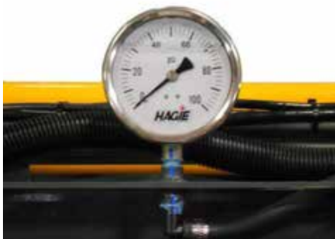
Pressure Gauge (Located on transom) -Typical View
