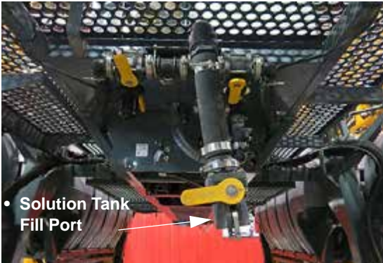
Rear Fill Assembly (Located beneath rear of machine) -Typical View
