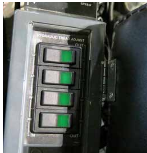
Hydraulic Tread Adjust Switches (Located near side console - open armrest to access) -Typical View
