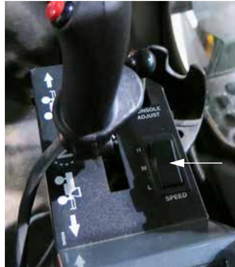
Speed Range Switch (Located near the Hydrostatic Drive Control Handle) -Typical View
