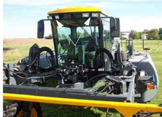
Field Lights (Mounted on the front of cab) -Typical View
