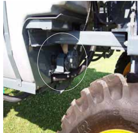
Agitator Motor (Located behind each solution tank) -Typical View
