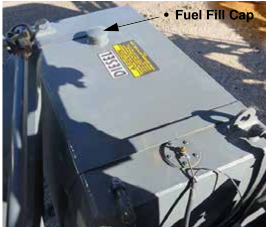
Engine Fuel Fill (Located on top of fuel tank on each side of machine) -Typical View
