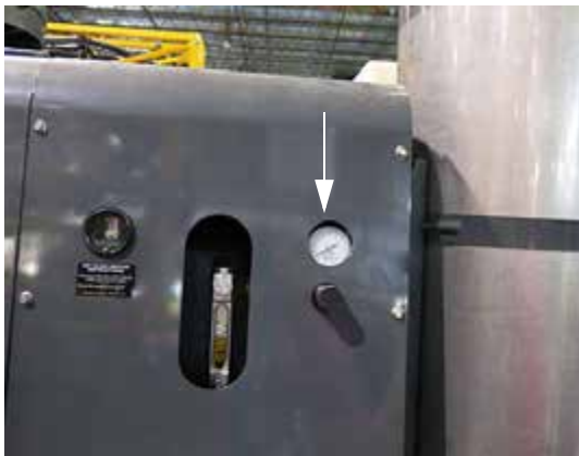
Foam Marker Pressure Gauge (Located near the rear left-hand side of machine) -Typical View
