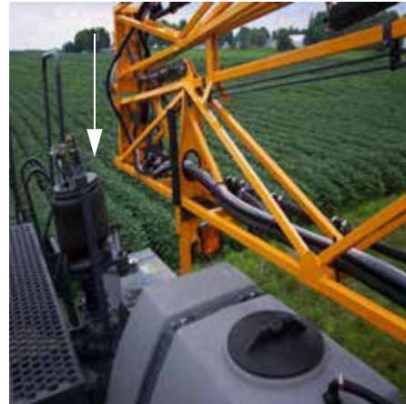
Lower boom level until full weight of boom is resting in cradle -Typical View
