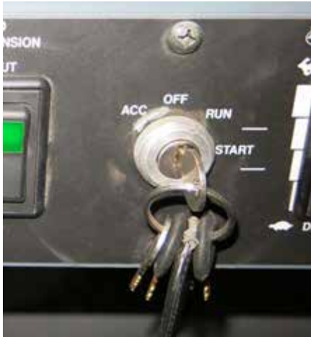
Ignition Switch (Located on the side console) -Typical View
