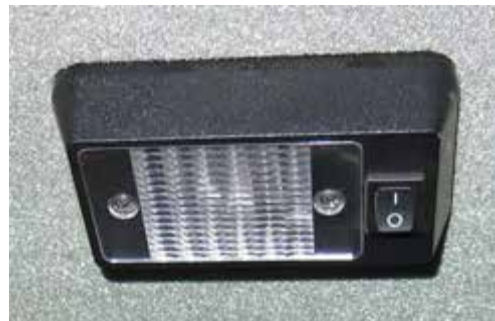
Interior Work Light (Located on cab headliner) -Typical View
