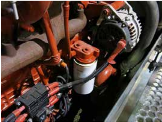
Engine Oil Filter (Located on the right-hand side of machine - open hood to access) -Typical View
