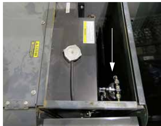
A/C System Receiver/Dryer (Located behind cab near the radiator - remove radiator screens to access) -Typical View
