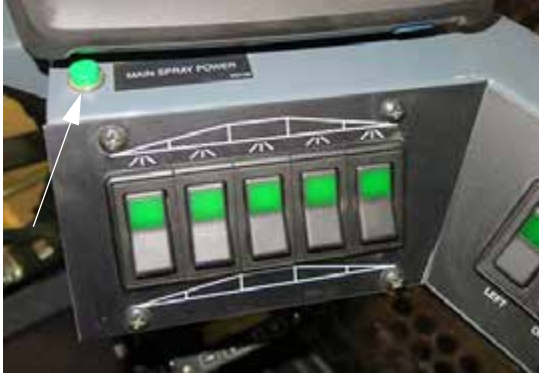
Master Spray Indicator (Located on the side console) -Typical View
