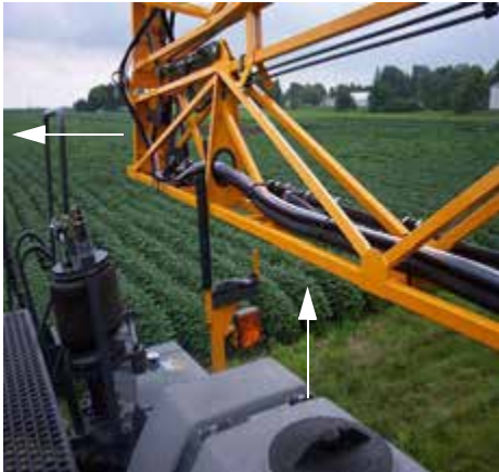
Raise boom level until it clears outer cradle stop -Typical View
