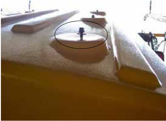
Roof Panel Mounting Bolts/Washers (Located on top of cab roof) -Typical View
