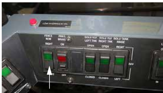
Fence Row Switch (Located on the side console) -Typical View
