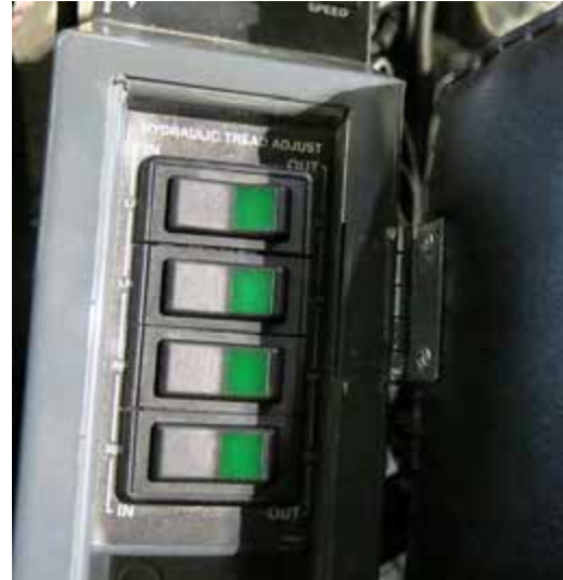
Hydraulic Tread Adjust Switches (Located near the side console - open armrest to access) - Typical View
