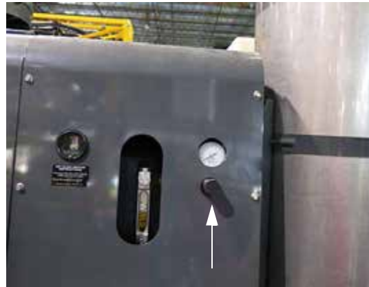
Foam Pressure Dial (Located near the rear left-hand side of machine) -Typical View
