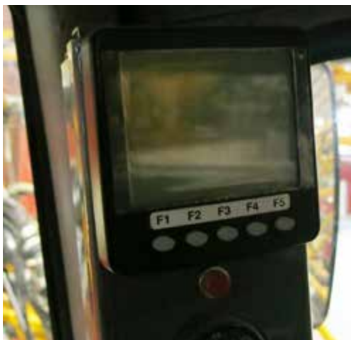
Engine Monitor (Located near the side console) -Typical View
