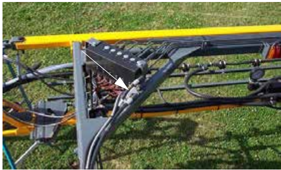
Boom Stack Valve -Typical View
