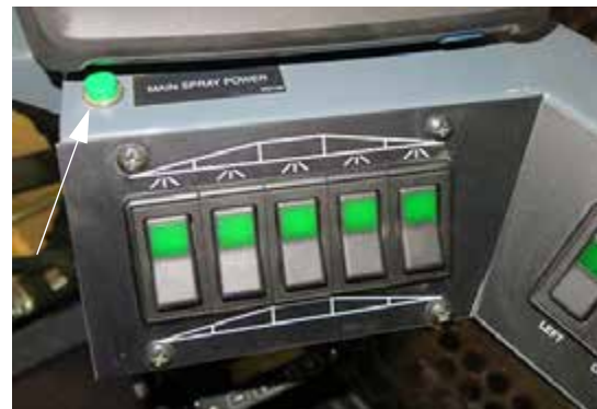
Master Spray Indicator (Located on the side console) -Typical View
