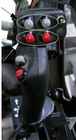
Left/Right Boom Level Switches (Located on the Hydrostatic Drive Control Handle) -Typical View
