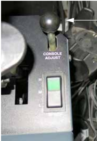
Console Adjust Lever (Located near Hydrostatic Drive Control Handle) -Typical View
