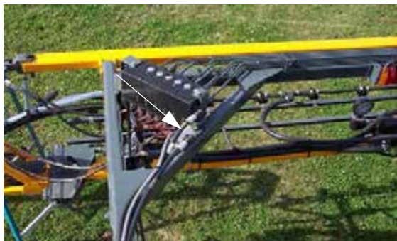
Boom Stack Valve -Typical View
