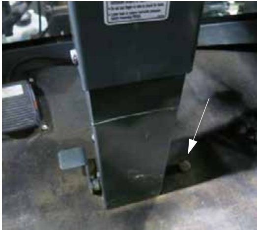
Master Spray Switch (Located on the lower right-hand side of steering column) -Typical View
