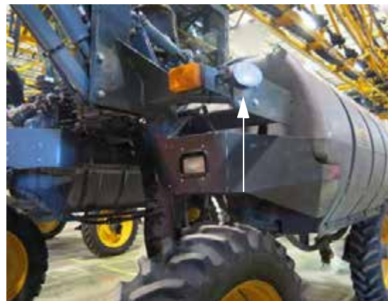
Work Lights (Located on the transom mount and rear of cab) -Typical View
