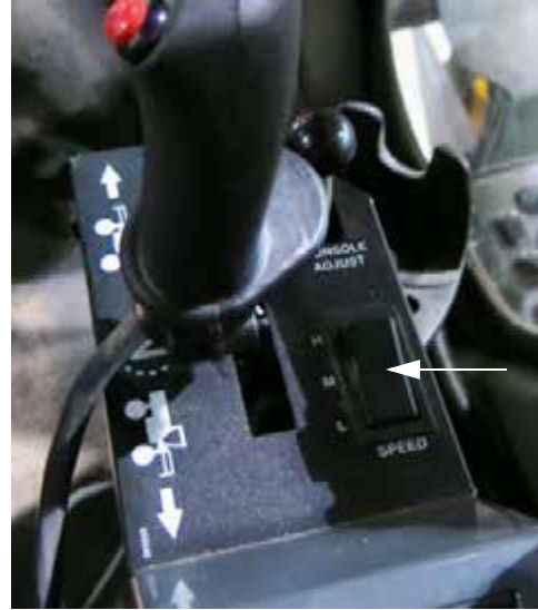
Speed Range Switch (Located near the Hydrostatic Drive Control Handle) -Typical View
