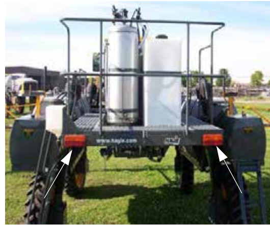
Running Lights (Located on rear of machine) -Typical View
