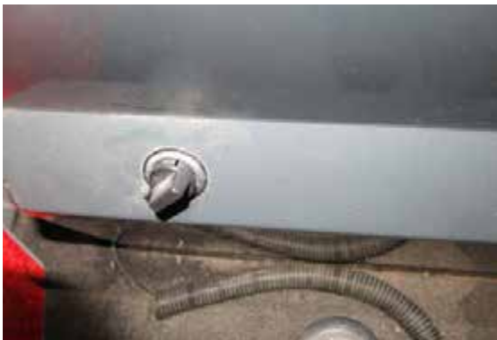
Power Port - Storage Console (Located on lower storage console on the left-hand side of operator's seat) -Typical View
