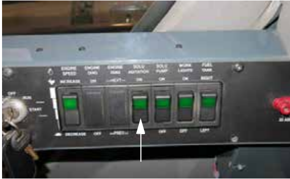
Agitation Valve Switch (Located on side console) -Typical View
