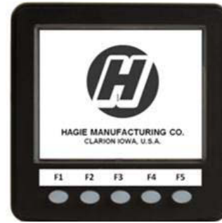
CANtrak Engine Monitor (Located near the operator’s station) -Typical View * Start-up screen shown
