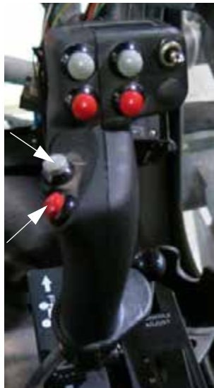
Transom Raise/Lower Switches (Located on the Hydrostatic Drive Control Handle) -Typical View
