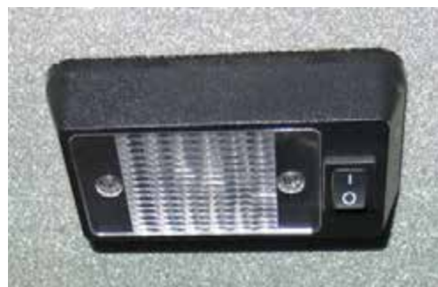
Interior Work Light (Located on cab headliner) -Typical View
