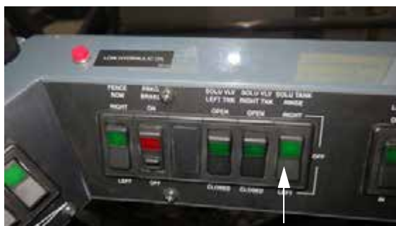
Rinse Switch (Located on the side console) -Typical View
