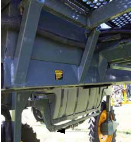
Rear Lock Nut (Located on leg brace) -Typical View
