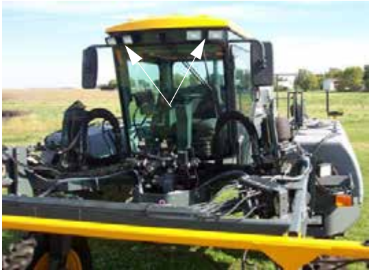
Field Lights (Mounted on the front of cab) -Typical View
