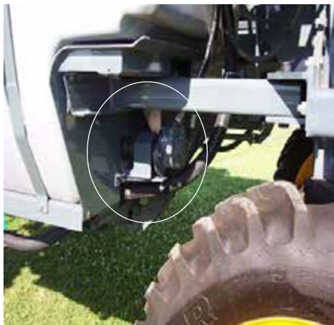
Agitator Motor (Located on each solution tank) -Typical View
