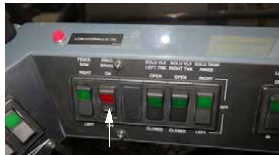
Parking Brake Switch (Located on the side console) -Typical View
