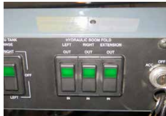
Boom Fold Switches (Located on the side console) -Typical View
