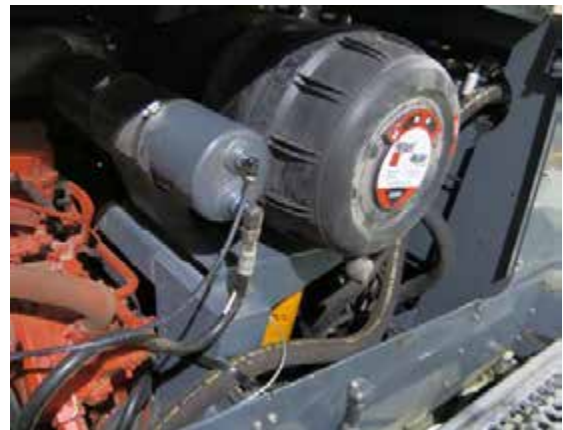
Engine Air Intake Filter (Located behind left-hand engine compartment) -Typical View
