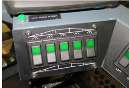
Boom Solution Valve Switches (Located on side console) -Typical View
