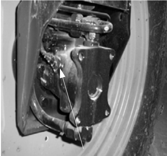
Speed Sensor (Located on the rear left-hand wheel motor) -Typical View
