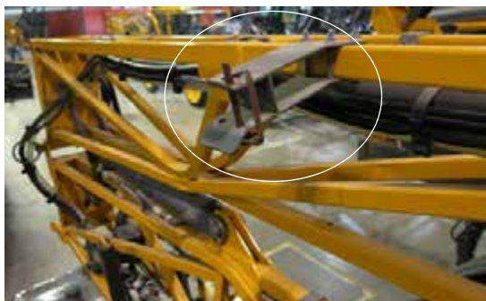
Lock Pin (Located near the rear of each folded boom extension) -Typical View
