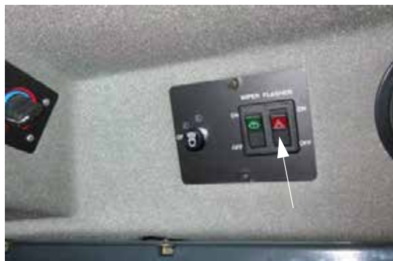
Hazard/Warning Lights Switch (Located on cab headliner) -Typical View
