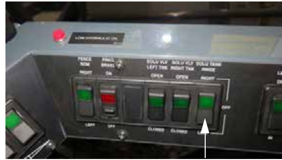
Rinse Switch (Located on side console) -Typical View
