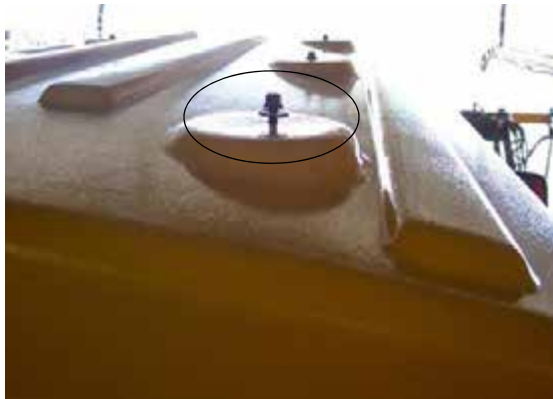
Roof Panel Mounting Bolts/Washers (Located on top of cab roof) -Typical View
