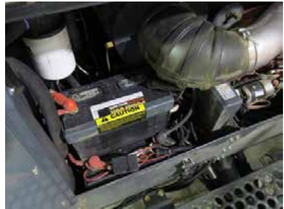
Battery Access (Located on the rear right-hand side of machine - open hood to access) -Typical View
