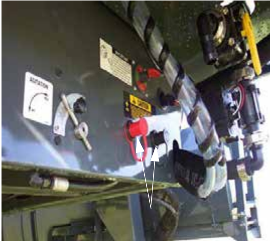
Auxiliary Battery Charging Posts (Located on the rear mainframe) -Typical View
