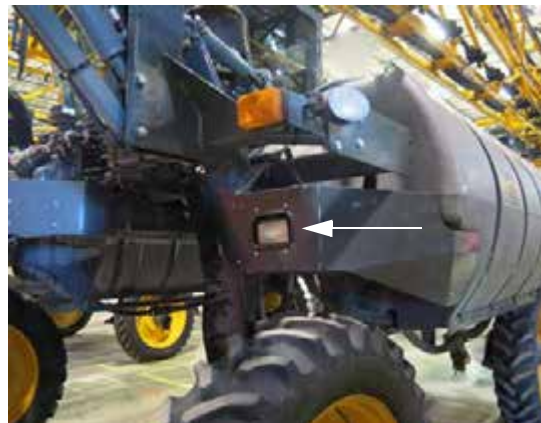
Highway Lights (Mounted on the center of each front tank shield) -Typical View
