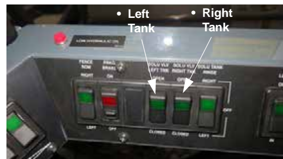
Solution Tank Valve Switches - Left/Right (Located on the side console) -Typical View
