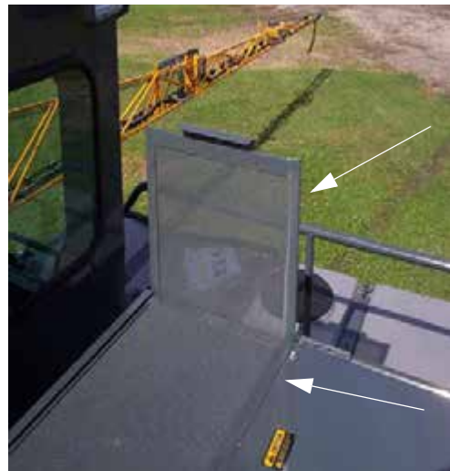
Radiator Screens (Located behind cab near the radiator) -Typical View
