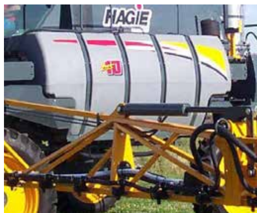
Solution Tank (Located on each side of machine) -Typical View
