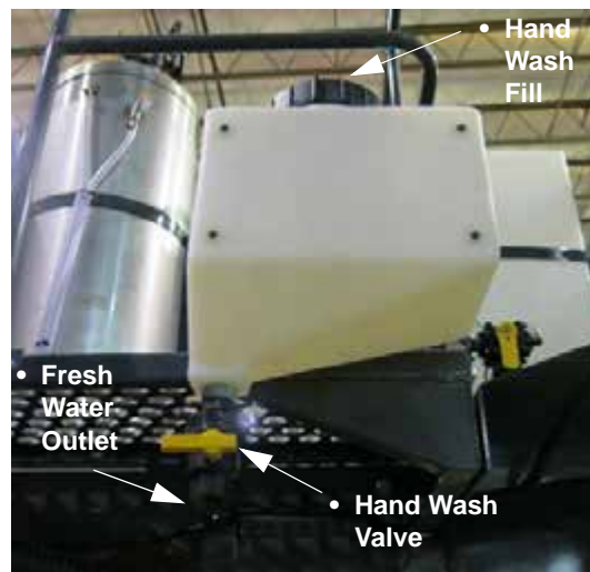
Hand Wash Tank (Located near rear left-hand side of machine) -Typical View
