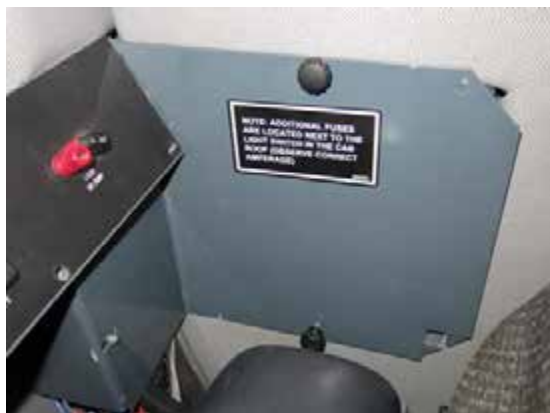
Fuse Panel (Located on the right-hand side of the operator's seat) -Typical View
