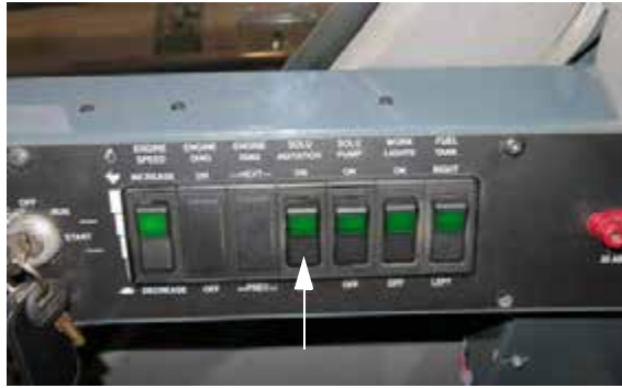
Agitation Valve Switch (Located on side console) -Typical View
