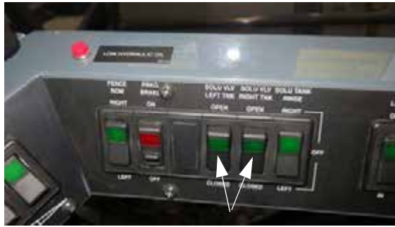
Solution Tank Valve Switches - Left/Right (Located on the side console) -Typical View
