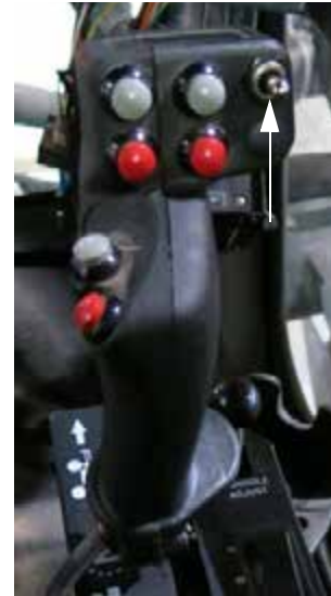
Foam Marker Switch (Located on the Hydrostatic Drive Control Handle) -Typical View
