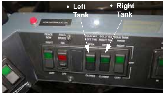
Solution Tank Valve Switches (Located on the side console) -Typical View
