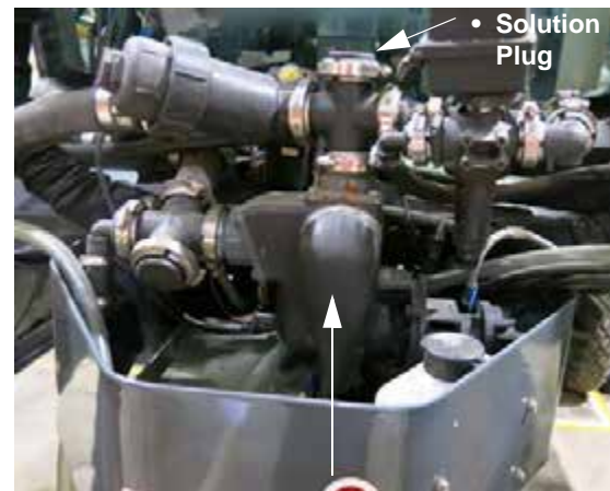
Solution Pump (Located near front of machine) -Typical View
