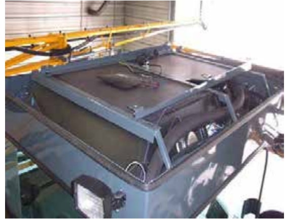
Roof Panel Removal -Typical View
