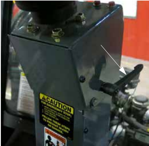
Tilt Lock Lever (Located on the right-hand side of steering column) -Typical View
