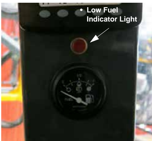
Fuel Gauge (Located near the side console) -Typical View
