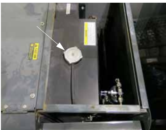
Radiator Cap (Located behind cab - remove radiator screens to access) -Typical View
