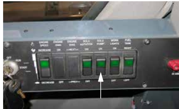
Solution Pump Switch (Located on side console) -Typical View
