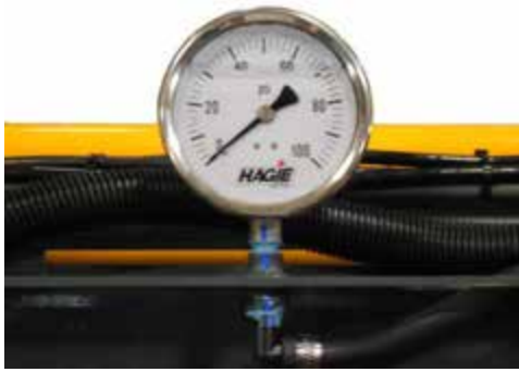
Pressure Gauge (Located on transom) -Typical View
