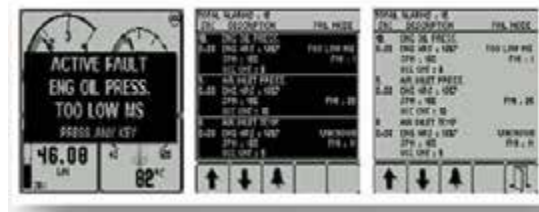
Active Alarm -Typical View
