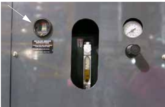
Filter Minder (Located near the rear left-hand side of machine) -Typical View
