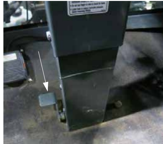
Steering Column Release Pedal (Located on the lower left-hand side of steering column) -Typical View
