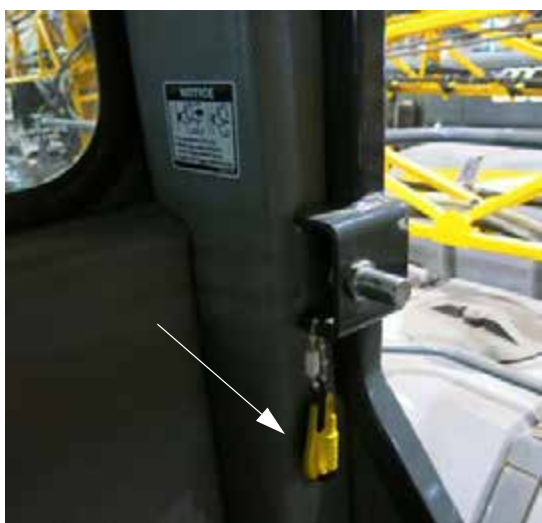
Emergency Exit Tool (Located on rear left-hand side of cab) -Typical View
