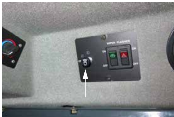
Field Lights Switch (Located on cab headliner) -Typical View
