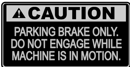
Near brake switch on switch panel in cab.
