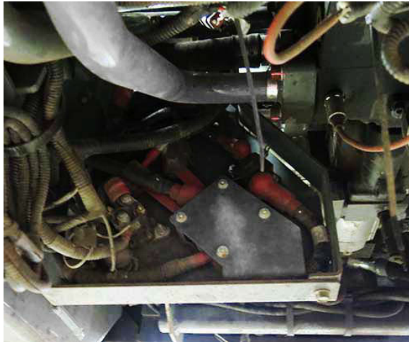
Final Tier 4 Engine Fuse/Relay Block (Located beneath batteries on the rear right-hand side of machine) -Typical View
