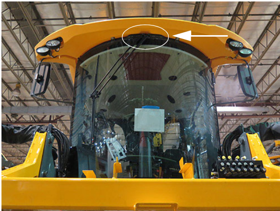
Windshield Washer Fluid Spray Nozzle (Located near top of exterior cab) -Typical View
