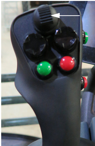
All Up/Down Switch (Located on the Hydrostatic Drive Control Handle) -Typical View
