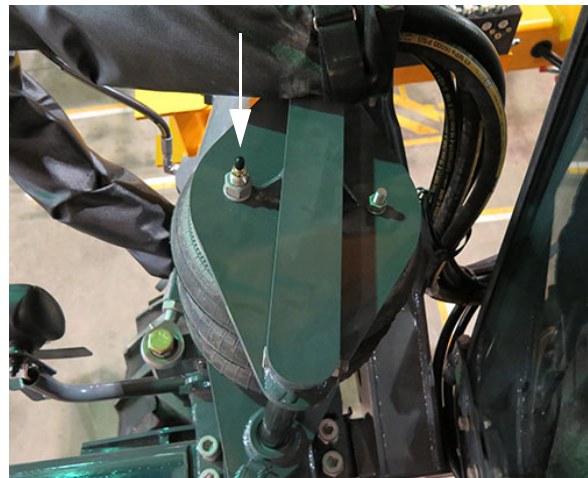
Air Bag Valve (Located on top of each air bag) -Typical View
