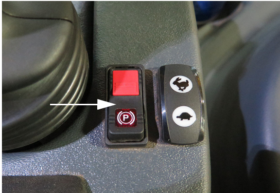
Parking Brake Switch (Located near the Hydrostatic Drive Control Handle) -Typical View
