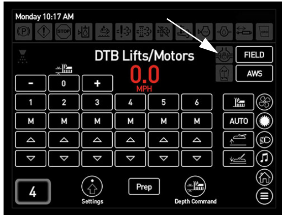
Traction Valve Indicator (Located on the Machine Display Home Page - Road and Field Mode) -Typical View
