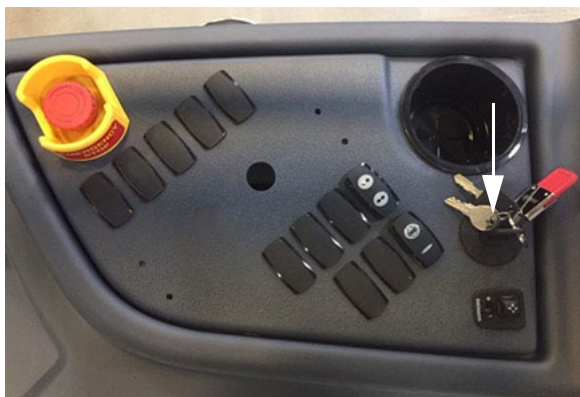
Ignition Switch (Located on the side console) -Typical View
