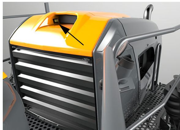
Hood Actuator Switch (Located near front of hood above the radiator screen) -Typical View
