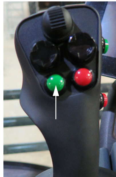
Main Motor Switch (Located on the Hydrostatic Drive Control Handle) -Typical View
