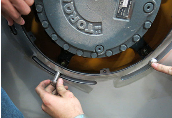
Wheel Cover Mounting Bolt Installation -Typical View
