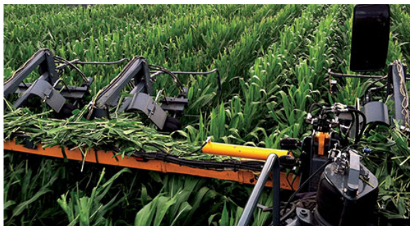
Detasseler Tool Bar (Shown with quad pullers) -Typical View
