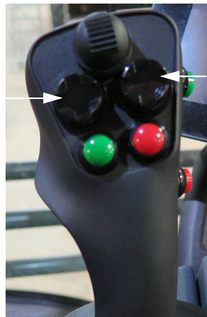
Outrigger Fold Switches - Left/Right (Located on the Hydrostatic Drive Control Handle) -Typical View
