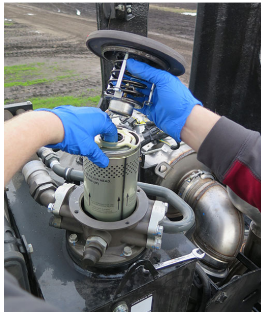
Return Filter 1 (Located inside filter housing on top of hydraulic oil reservoir - open hood to access) -Typical View
