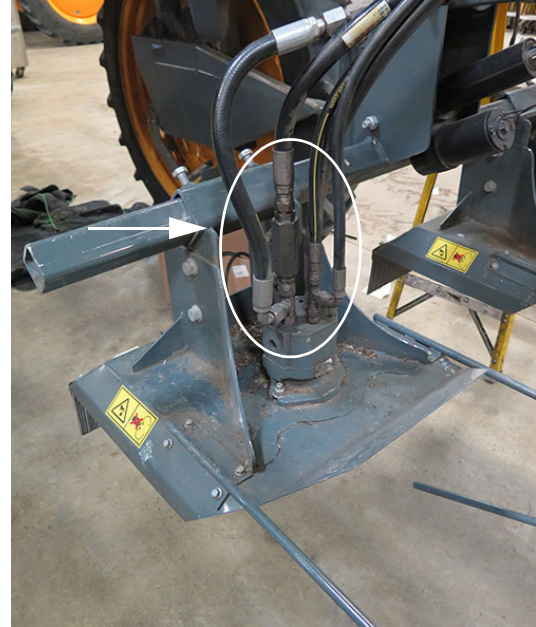
Cutter Head Hydraulic Connections -Typical View
