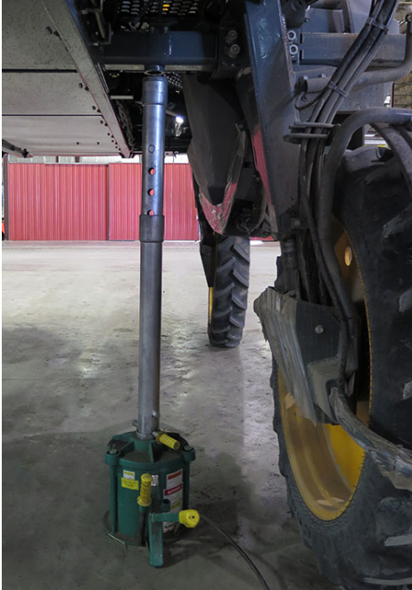
Align Jack with Lifting Point Containment Ring -Typical View
