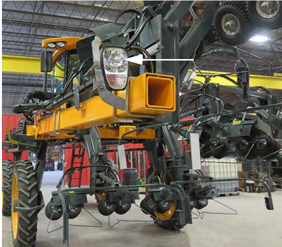
Highway Running Lights (2) -Typical View
