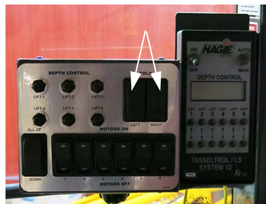
Outriquer Fold Switches - Left/Right (Located on the detasseling control panel) -Typical View
