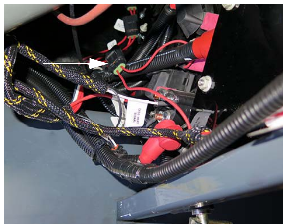
Hood Actuator Fuse (Located beneath rear right-hand side of machine) -Typical View
