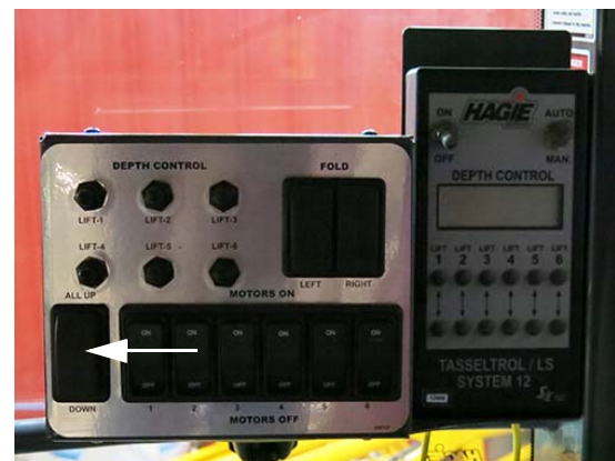
All-Up/Down Switch (Located on the detasseling control panel) -Typical View
