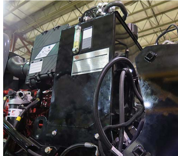
Hydraulic Oil Reservoir (Located near rear left-hand side of machine - open hood to access) -Typical View
