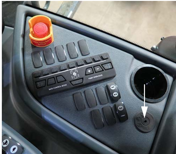
Ignition Switch (Located on the side console) -Typical View
