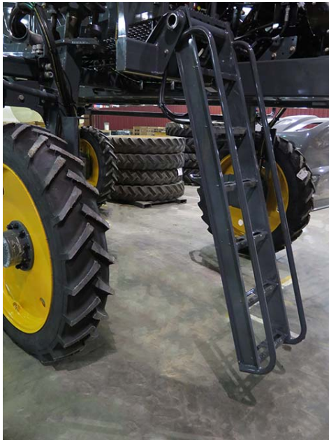
Ladder -Typical View * Lowered position shown
