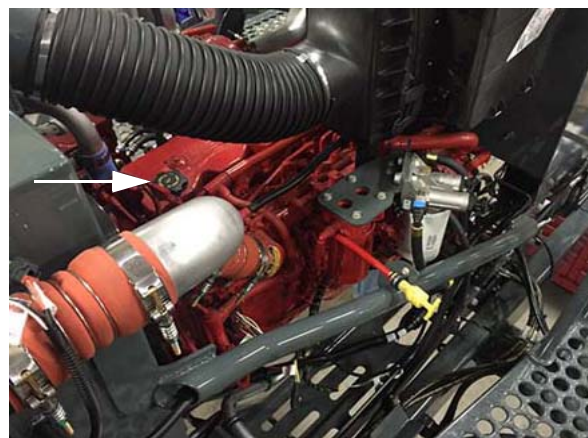
Engine Oil Fill (Located near top of engine - open hood to access) -Typical View
