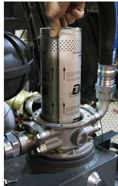
Return Filter 1 (Located inside filter housing on top of hydraulic oil reservoir - open hood to access) -Typical View
