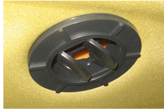
Cab Vent -Typical View
