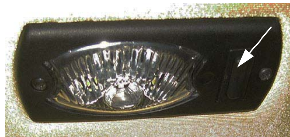
Interior Work Light Switch -Typical View
