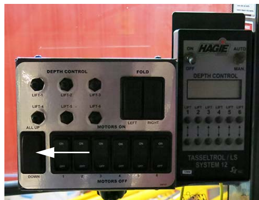
All-Up/Down Switch (Located on the Detasseling Control Panel) -Typical View
